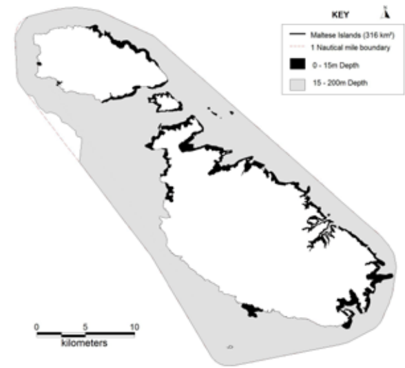
Figure 1: The grey area depicts the bathymetric sidescan zone, the black depicts the bathymetric LIDAR zone and the white depicts the terrestrial LIDAR zone.
