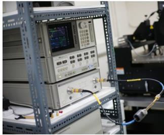
HP 20 GHz RF Network Analyser measuring S-parameters of a microstrip filter
