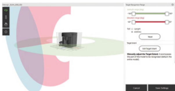
Figure 1. Model target-generation via Vuforia's deep learning techniques
