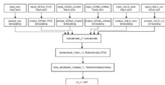
Figure 2. Structure of the Bi-LSTM-CRF model in Keras
