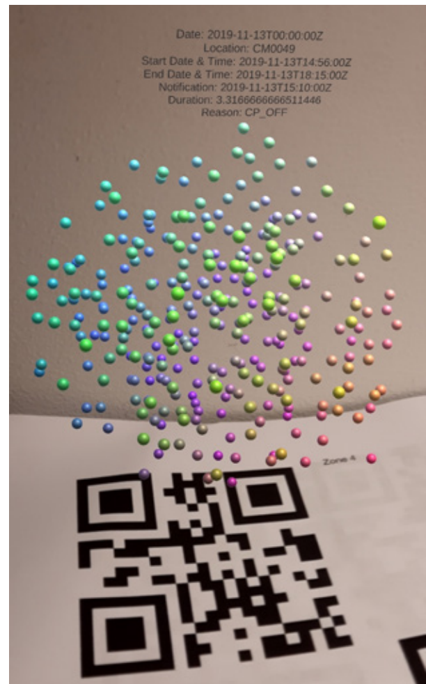
Figure 2. Diagram of the AR application, displaying the 3D scatterplot for a zone showing single-point data
