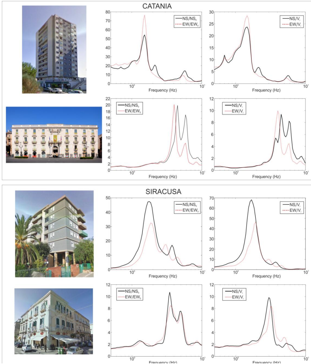
Figure 1. Examples of HVNR and SNSR for typical RC and MA buildings in Catania and Siracusa. The y-axis specifies the amplitude ratio.
