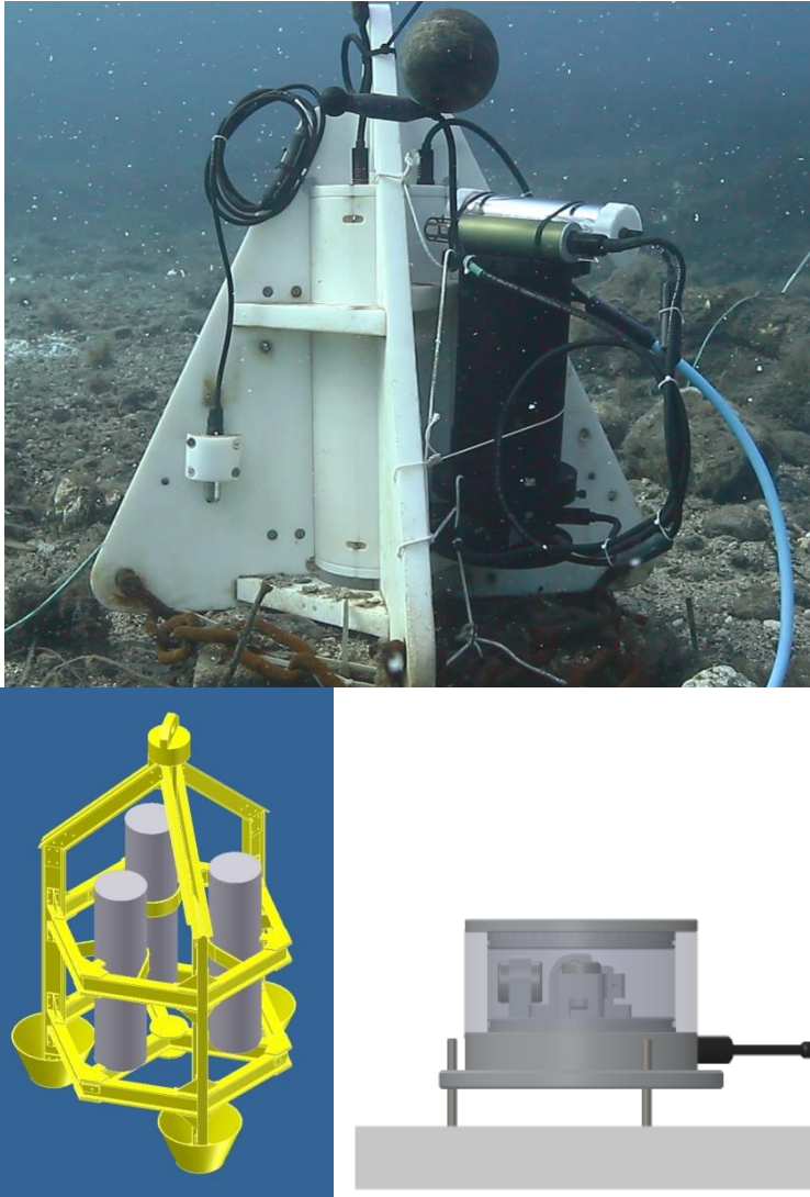
Figure 2: The sea-floor observatory deployed off the island Panarea at shallow depth. The picture shows two observatories contemporary working and connected to same cable. The black vessel contains the electronic devices that will feed the seafloor observatory developed in MONSOON project. There are three probes connected: the dissolved CO 2 (white probe, digital output), a hydrophone and the very sensitive temperature probe from Sea-Bird (bronze probe, analog output). The geophone will be connected to the same electronic cards. (bottom panel) Schematics of the sea-floor observatory and the geophone integrated in a vessel able to work at a depth of 2000m. The heavy platform is necessary to couple the geophone with the sea-floor. The geophone is equipped with an electronic compass and an system to check the tilt
