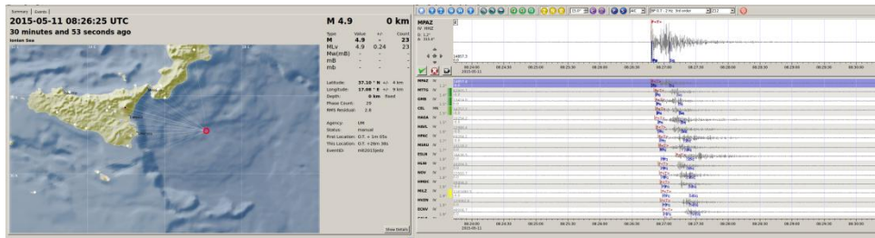
Figure 2. Screen shot of SeisComP3 graphic user interface showing the location of an earthquake (red circle on map) and the corresponding seismograms (right). Each trace is from a station shown as a coloured diamonds on the map, connected with a fine white line to the epicentre.
