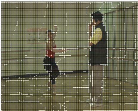
Fig. 9. MB partitions depending on the 8×8 changes in the depth map.
