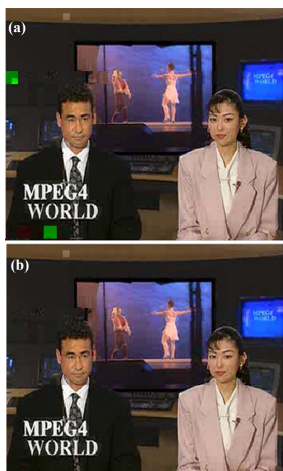
Fig. 5 Frame 8 of a corrupted Akiyo Sequence using (a) the standard H.263+ Decoder (b) the enhanced H.263+ Decoder with the spatial dissimilarity metric.
