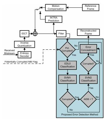
Fig. 1 Proposed Error Detection Algorithm
