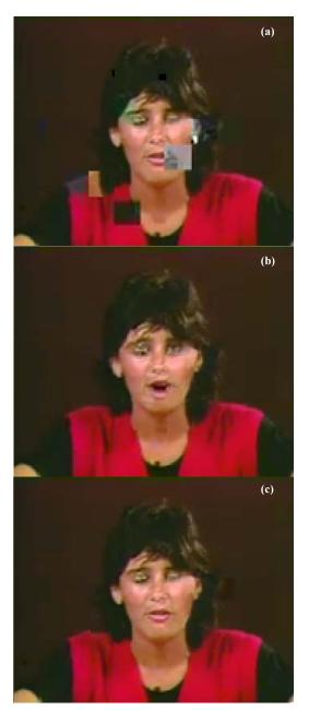
Fig. 6 Miss-America using (a) MB level concealment, (b) Slice Level Concealment, and (c) Proposed Error Detection method
