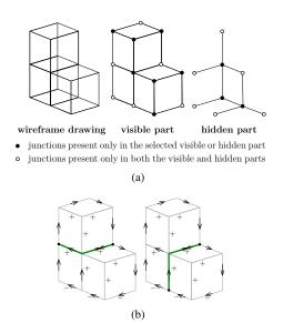
Fig. 3. (a) A wireframe drawing can be divided into a visible part and a hidden part. (b) Two SP paths in the drawing are shown.
