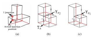
Fig. 2. (a) Showing the sketched T junction and its actual position in the wireframe drawing (b), (c) Drawings exhibiting an extended trihedral geometry, showing the separable edge labels and the Separable Y and T junctions.
