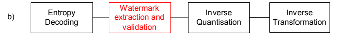
Figure 1: a) watermark insertion and extraction at the encoder, b) watermark extraction and validation at the decoder
