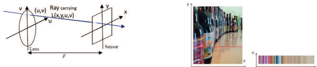
Fig. 1: (left) Illustration of the two planes parameterization of the 4D static (one time instant) light field; (right) Rendered image at one focus; and epipolar image corresponding to horizontal red line in left image.
