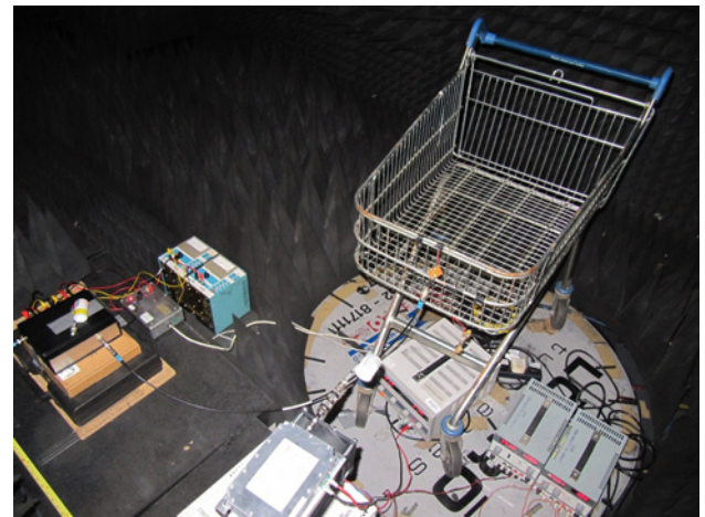
Fig. 11 Shopping trolley eavesdropping arrangement
