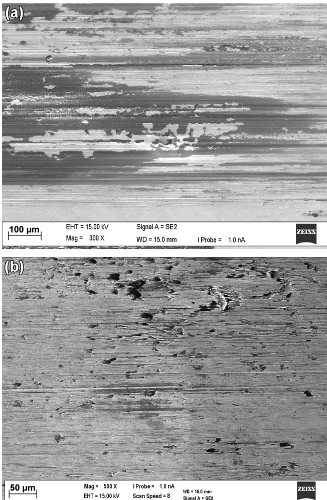
Fig. 14. SEM images of wear morphology on (a) ASTM F1586 carburised disk and (b) AISI 316 carburised ball tribopair (C500|C500). Direction of sliding: left to right.
