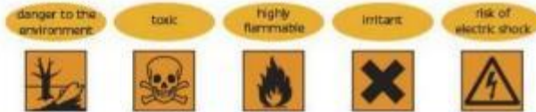
FIGURE 1: Hazard-warning signs. Can you think why they don't have any writing on them? (Hint: Imagine you were working in a laboratory in Russia and you didn't speak the language.)
