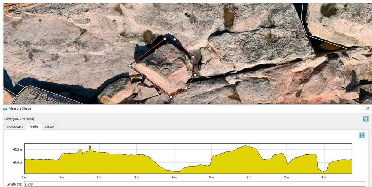
Figure 6. Polygon tool used to calculate the boulder surface area and volume using the Agisoft functionality.
