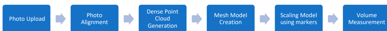
Figure 7. Workflow for the creation of individual boulder models on Agisoft Metashape for volume calculation.
