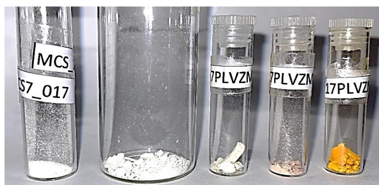
Figure 6.2. Change in colouration from the white coloured original MCS7_017 and drug loaded MCS7_077, and the cream coloured MCS7_080, pink coloured MCS7_082 and orange coloured MCS7_085, from conjugation of pH, electro, and UV responsive smart molecules respectively (left to right).
