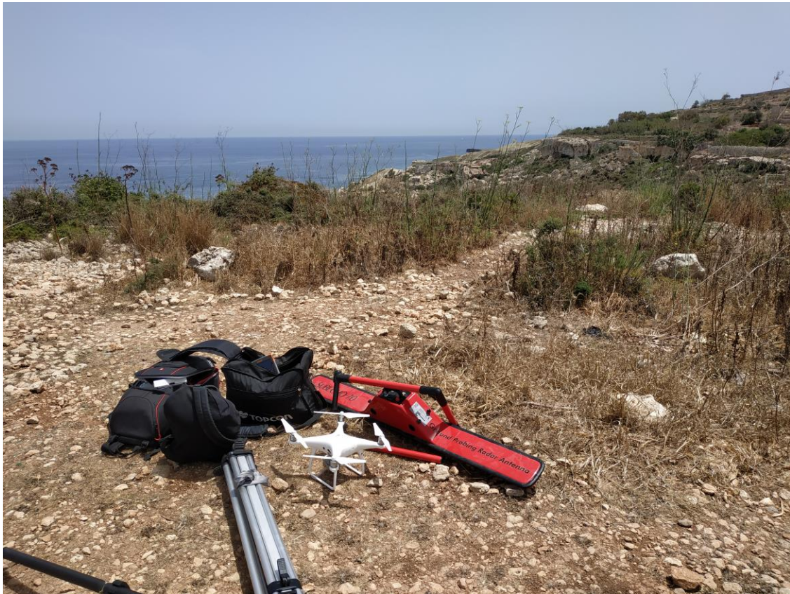
Figure 36: Photo acquired during the georadar survey. The photo shows the tripod and rod of the Differential GNSS, the Phantom 4 Pro UAV used for photogrammetric survey and the Cobra Subecho-70 georadar.
