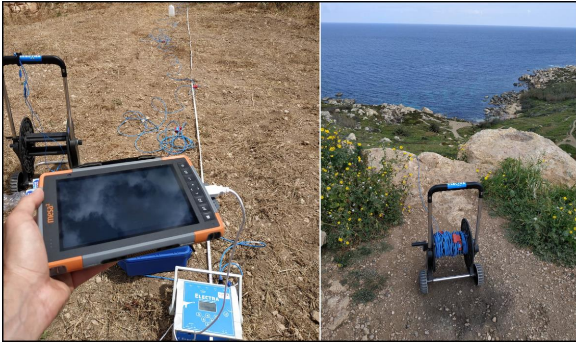
Figure 27: ERT data acquisition in Selmun (Malta) using a georesistivimeter model ELECTRA, from Moho Srl.
