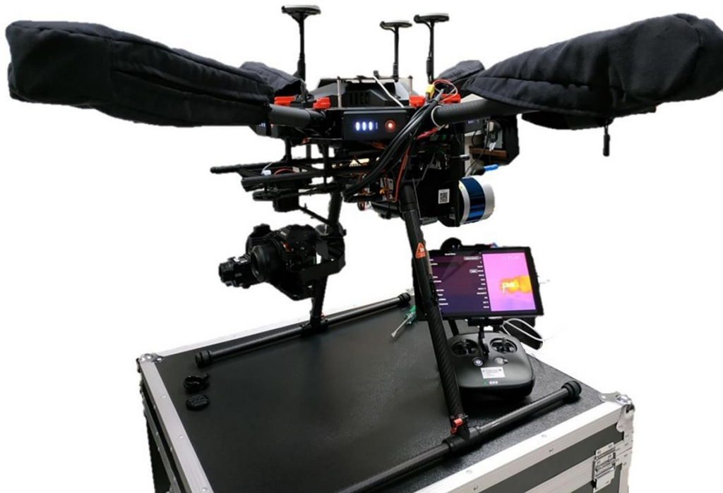
Figure 16: Hexacopter DJI M600 Pro equipped with LiDAR, thermal camera and RGB camera.
