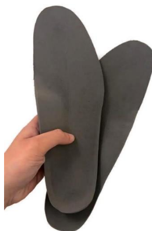
Figure 6 Illustrates a photo of one of the EVA insoles made with High Density EVA for one of the participants
