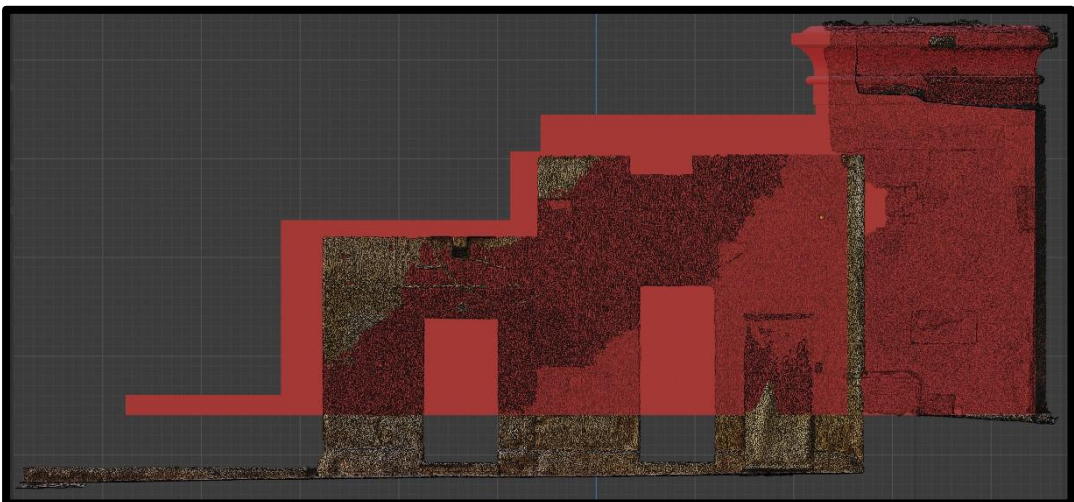
Figure 117. Screenshot from Blender showing the results of the comparative analysis: different results concern the heights of the two walls where the interpretative model (red mesh) has a wall located at a higher level than the reality-based one (black mesh) (photo by the author).
