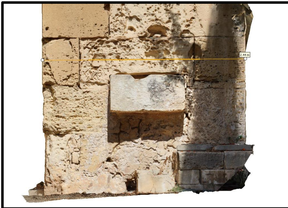
Figure 108. Screenshot from Agisoft Metashape showing the measured length of the tower from the reality-based 3D model using the 'ruler' tool (photo by the author).
