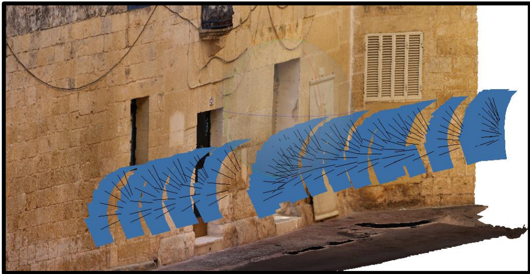
Figure 99. Screenshot from Agisoft Metashape showing the location of the hand-held camera pictures photogrammetrically surveying the wall alignment from Triq Karmnu (photo by the author).
