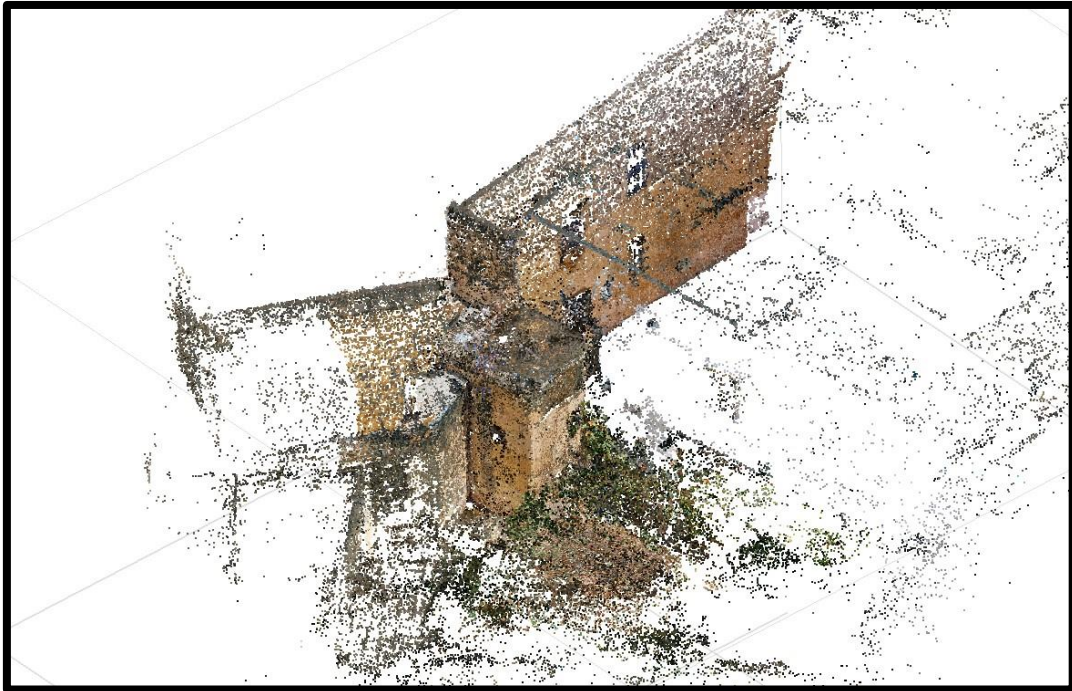
Figure 103. Screenshot from Agisoft Metashape showing the cloud of points of the reality-based 3D model (photo by the author).
