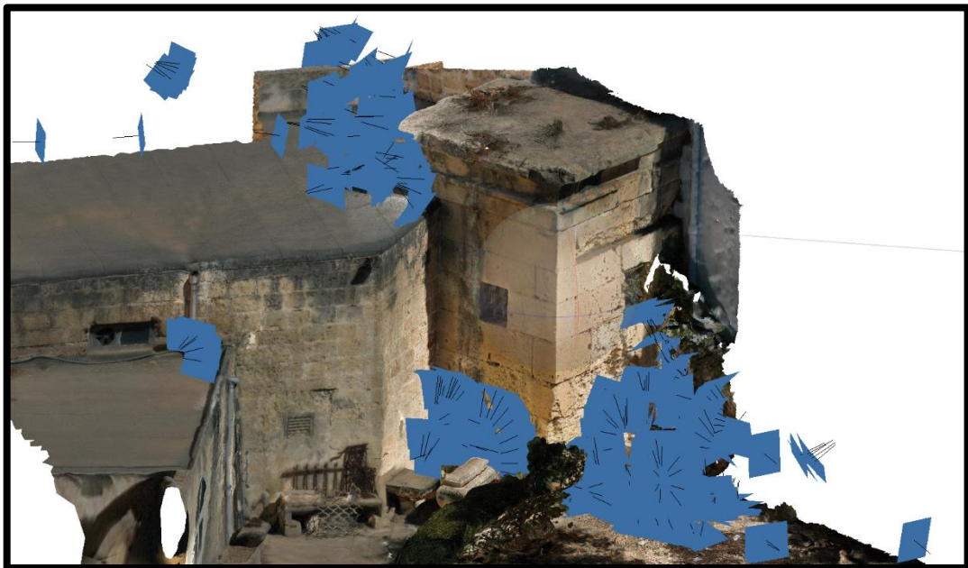
Figure 100. Screenshot from Agisoft Metashape showing the location of the hand-held camera pictures photogrammetrically surveying the tower from the garden of the Parish Office (photo by the author).
