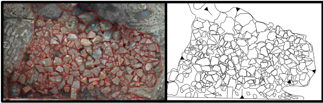
Figure 7. Image showing the plan drawing of an orthophotomosaic on a CAD software. (Image by the author).
