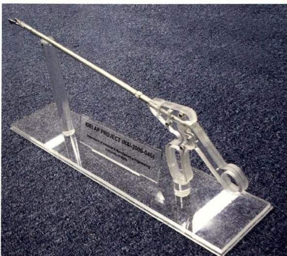
The prototype developed by the University research team incorporating scissors, the grasper and the hook in one tool
