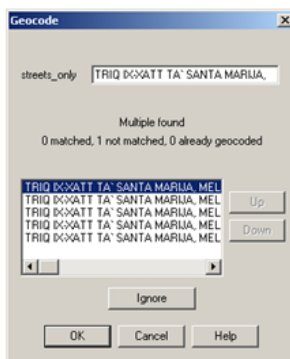
Figure C.10: Checking attribute data for matching to centreline through manual or automatic means
