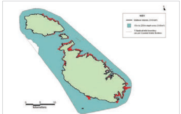
Fig 3: Total area scanned the blue area depicts bathymetric sidescan, brown bathymetric LIDAR, and green terrestrial LIDAR zones
