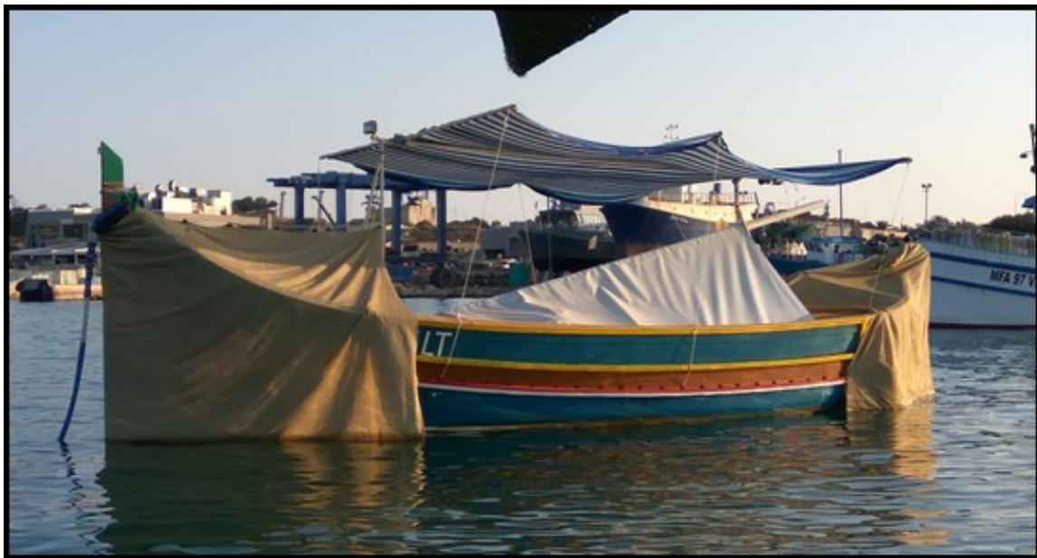
Picture 74: A luzzu fitted with an awning to protect against the damaging fresh water from rain and dew, and fitted with cloth to soak it with sea water which protects it against excessive dryness
