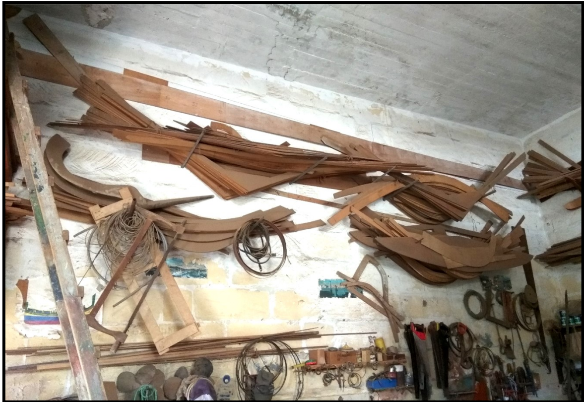
Picture 20: The boat frame templates (m. galvijiet ) still hanging at the Caruana's family workshop even though long retired. (Source: my own)
