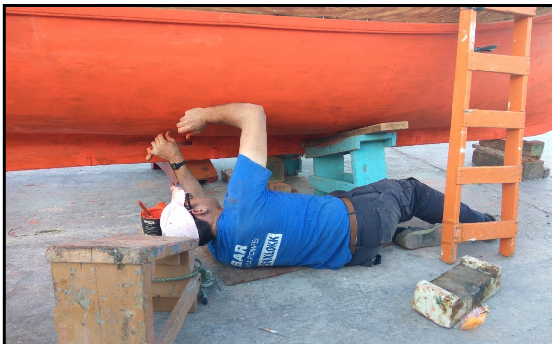
Picture 73: Applying wood putty to the openings with a chisel (Source: my own)
