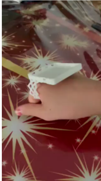
Figure 5.16: Testing the model of the main controller board. The board was too large so when the user made a fist or moved the wrist downwards, the board did not maintain constant contact with the back palm, meaning the motion sensor on it would not have given accurate readings
