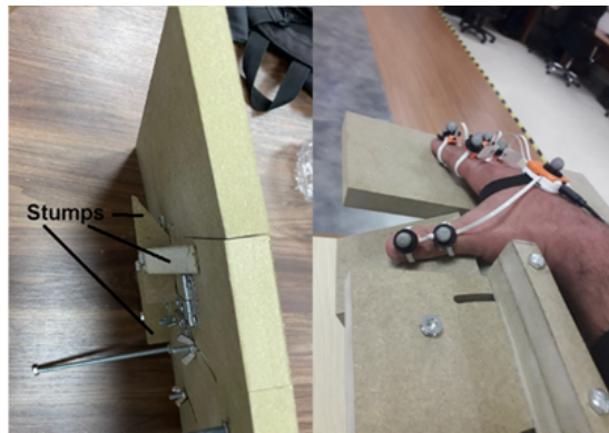
Figure 7.8: Stumps to set maximum bending angle (right) and an example with the thumb(left).
