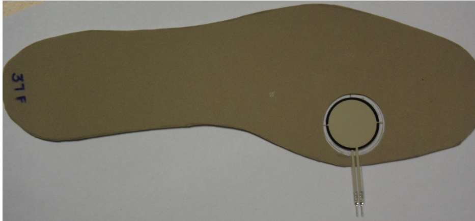
Figure 60: Photograph showing an example of simple insole used to hold the FSR sensor of the prototype over the FScan™ sensor insert
