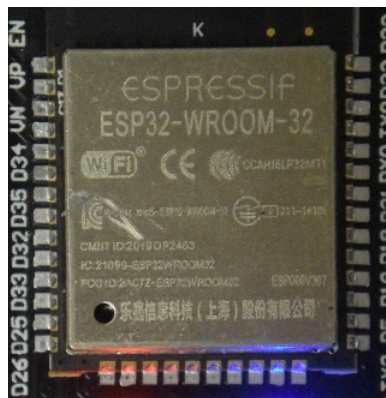
Figure 36: Photograph of the ESP23 type of microcontroller used
