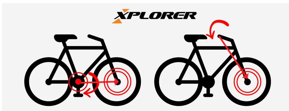
Figure 2.16 Diagram showing the difference in power control between pedelecs and powered cycles
