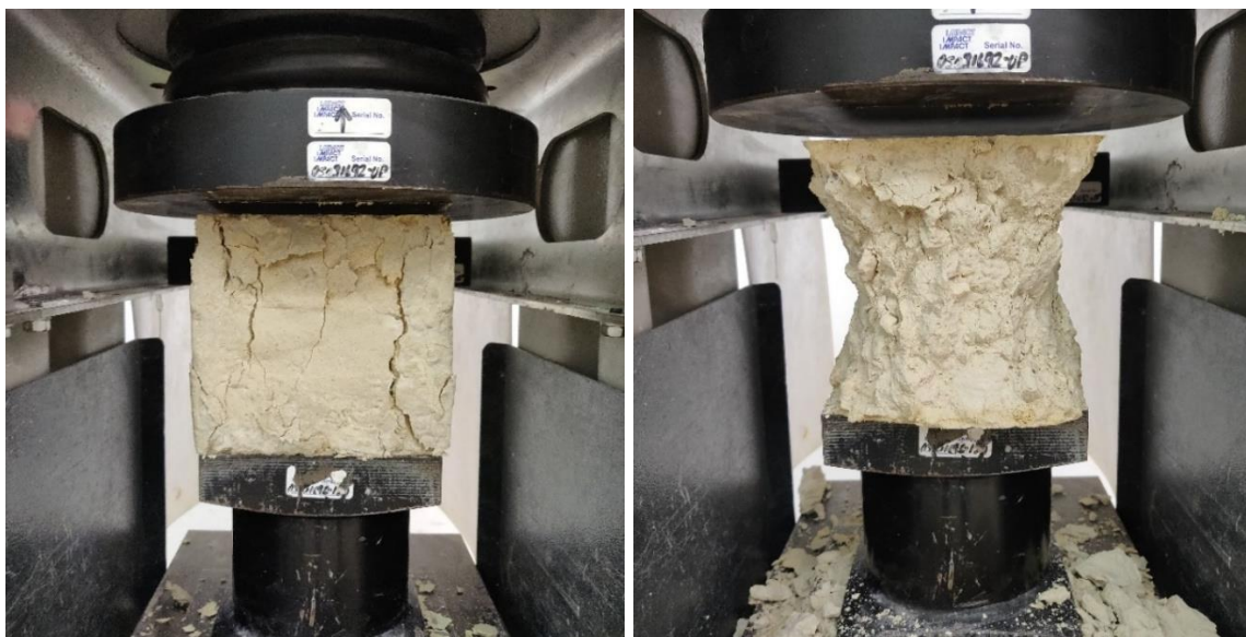
Figure D.4 – Typical Failure Mode for a concrete cube sample of batch 2
