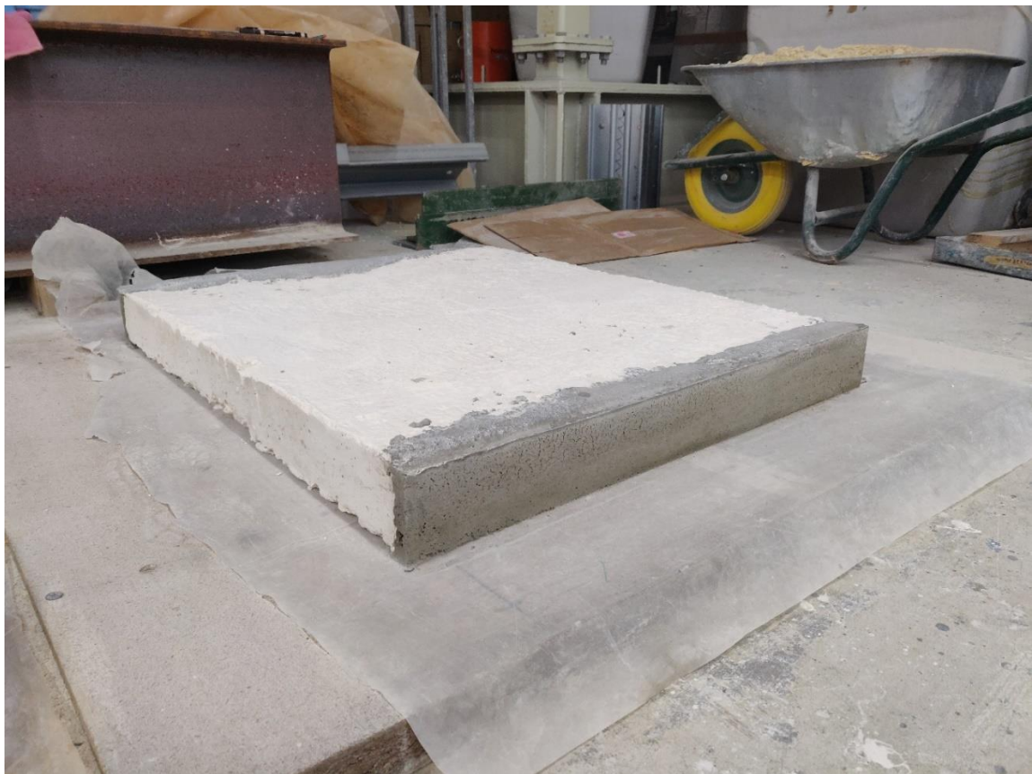
Figure G.3 – Grouting surface finish post curing
