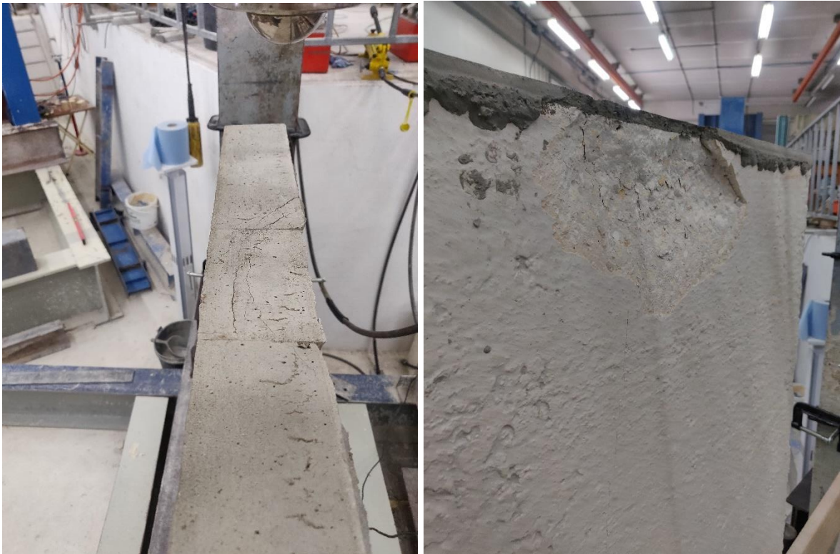
Figure F.41 – Concentrated load failure mode through the grout layer
