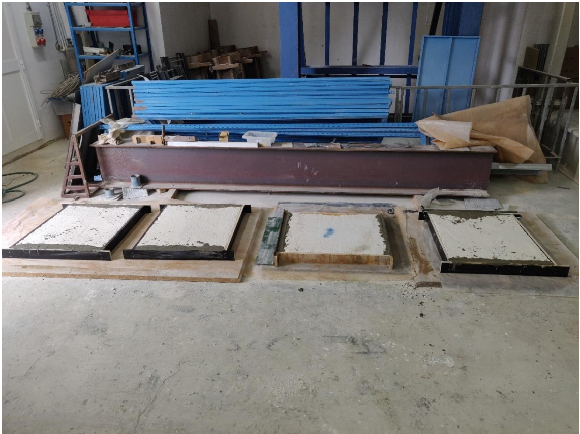
Figure G.2 – Grouting of the walls' loading surfaces
