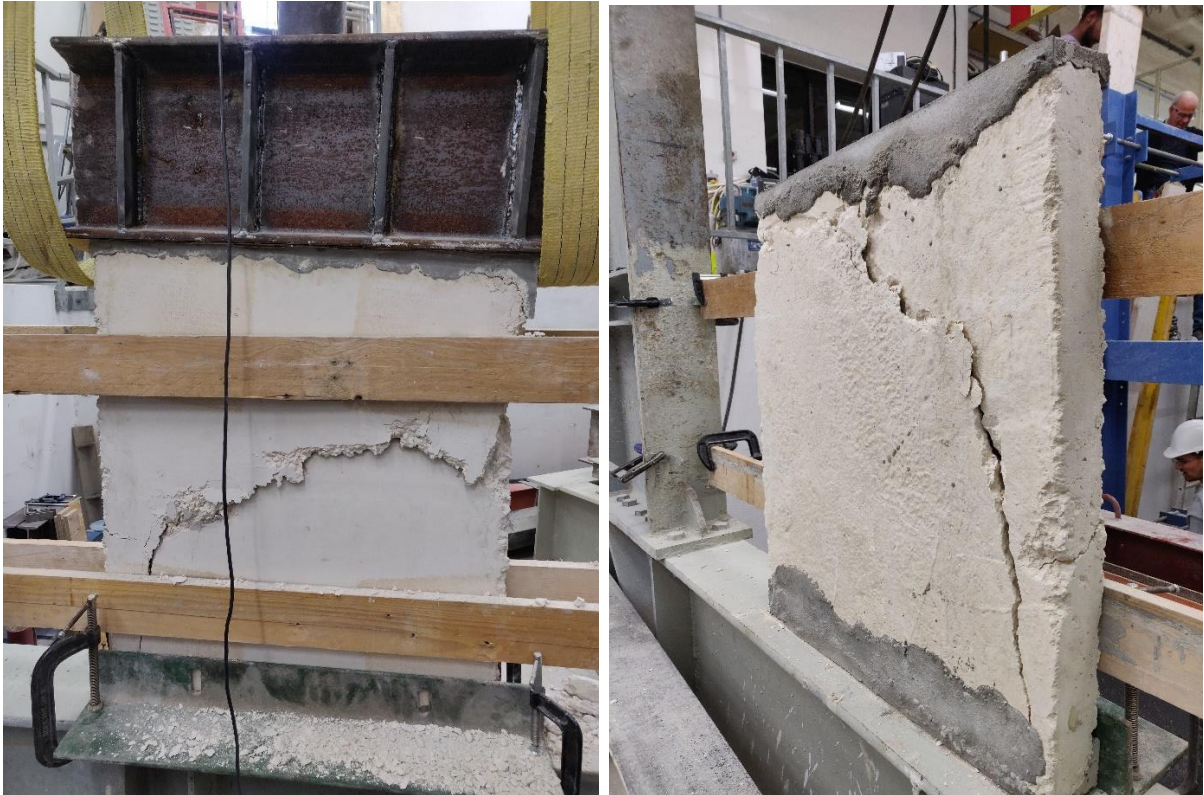
Figure 4.4 – Left , failure mode front elevation; right , failure mode back elevation
