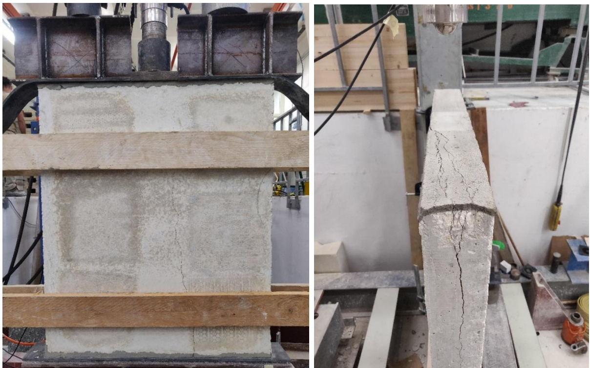
Figure 4.55 – Left , failure mode front elevation; right , failure mode underneath the left loading beam
