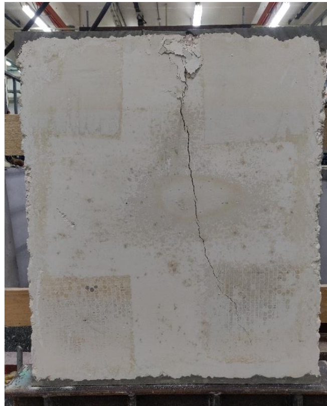
Figure 4.11 – Failure mode front elevation
