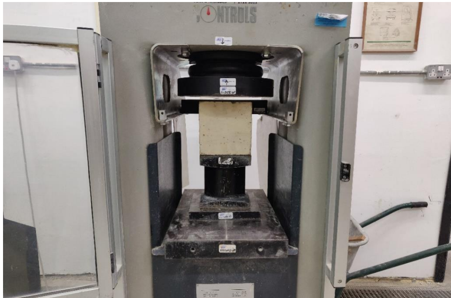
Figure D.3 – Typical Concrete cube from the second batch being tested
