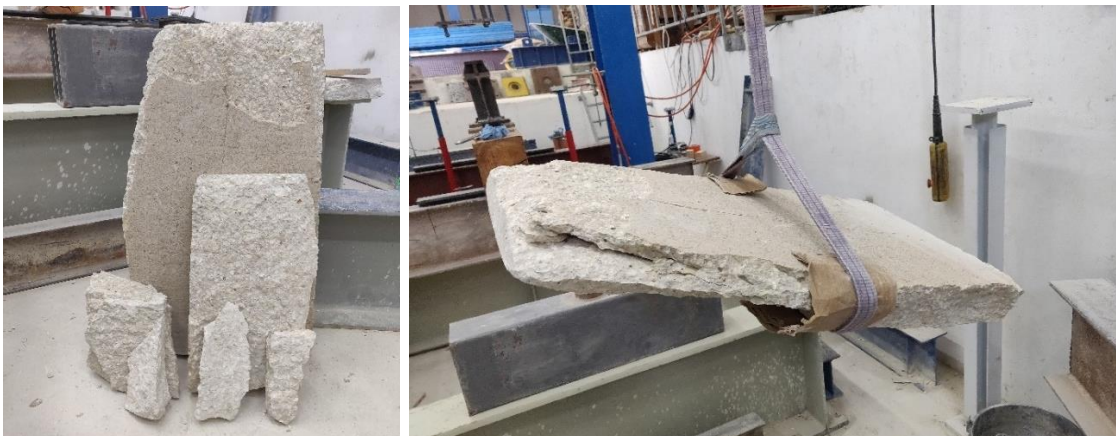
Figure F.29 – Left , left over pieces from the explosive failure; right , main vertical crack
