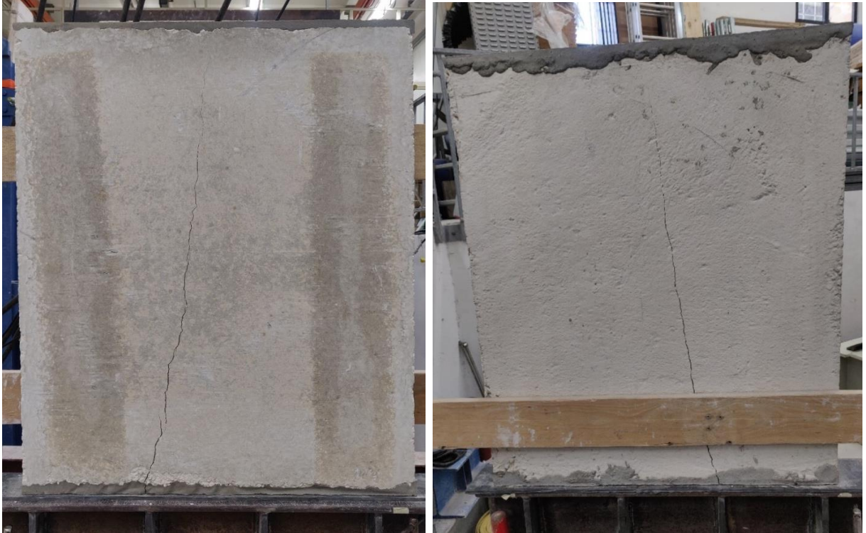
Figure 4.47 – Left , failure mode front elevation; right , failure mode back elevation
