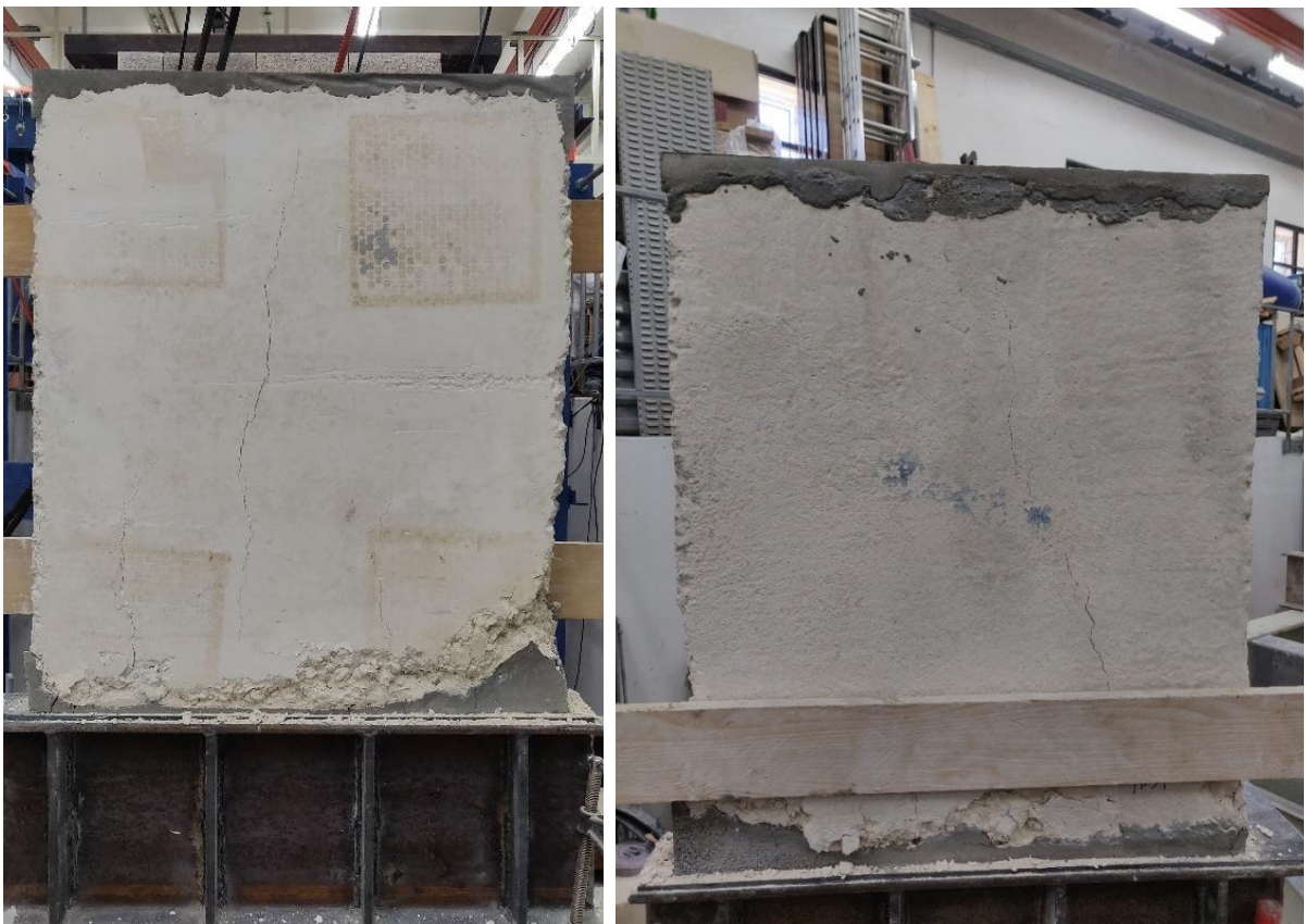
Figure 4.29 – Left , failure mode front elevation; right , failure mode back elevation
