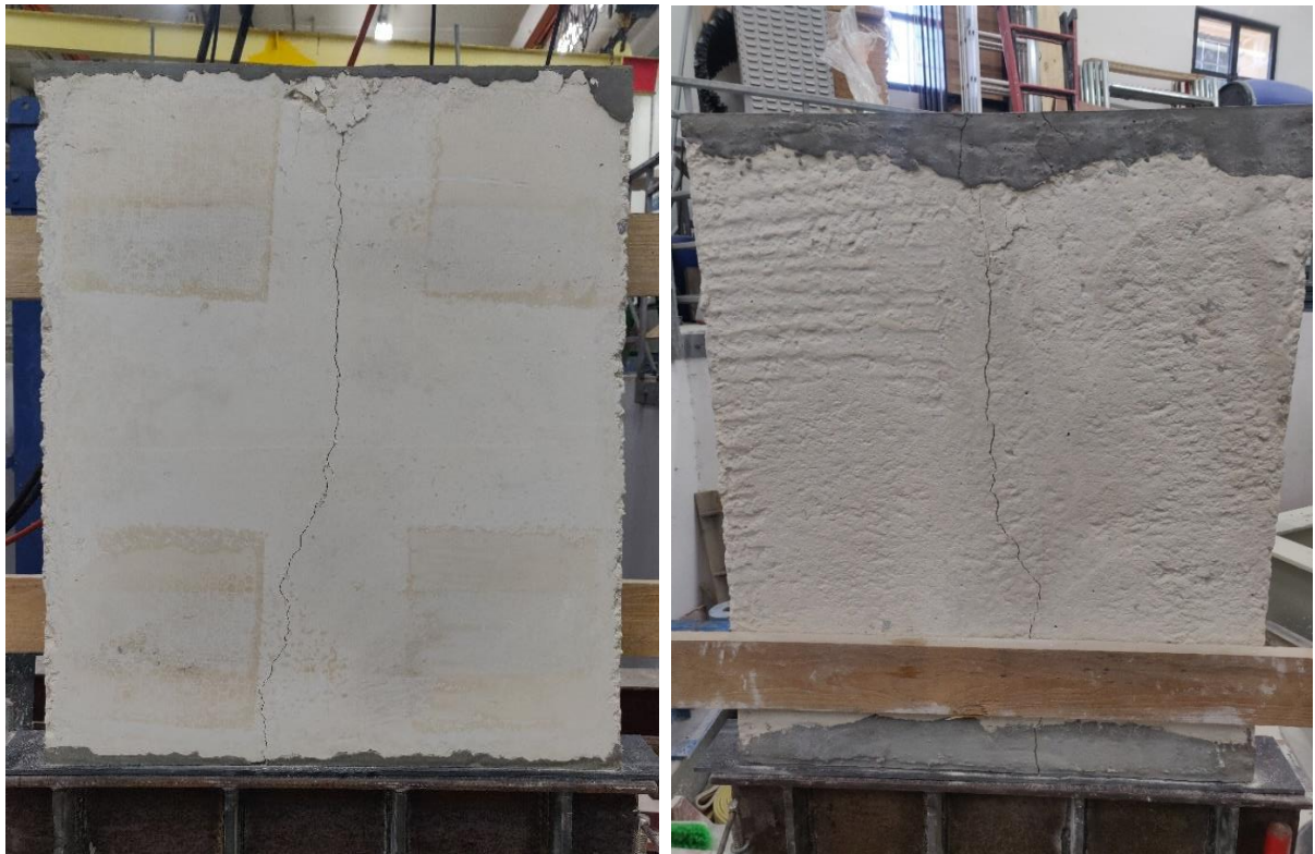
Figure 4.17 – Left , failure mode front elevation; right , failure mode back elevation
