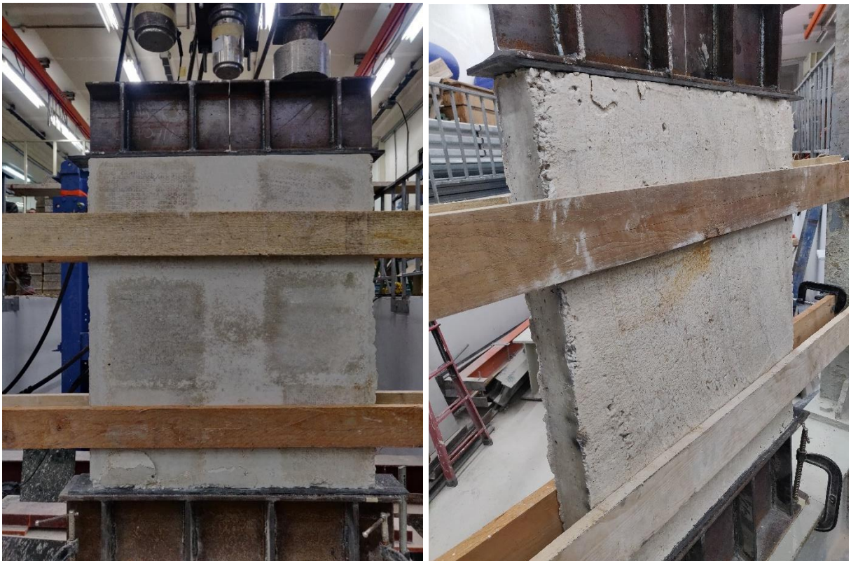
Figure 4.34 – Left , failure mode front elevation; right , failure mode back elevation
