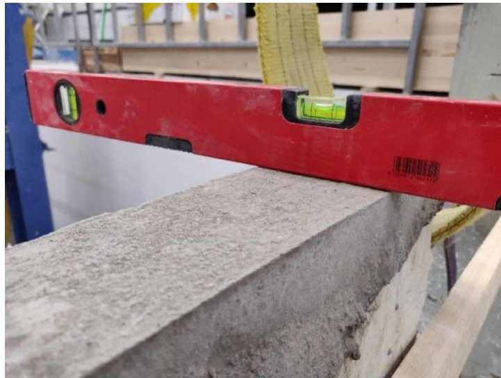
Figure 3.17 – Ensuring the loading surface is perfectly aligned using a spirit leveler
