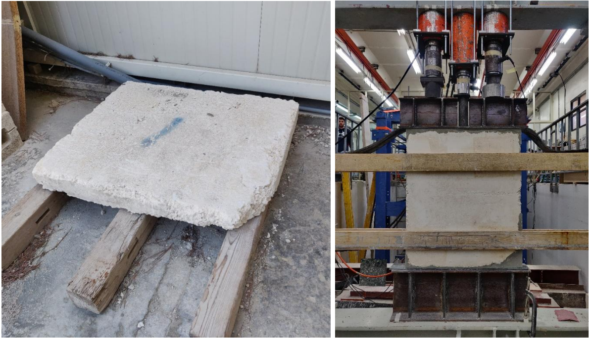
Figure 4.28 – Left ; damaged wall pre-grouting; right , repaired wall setup
