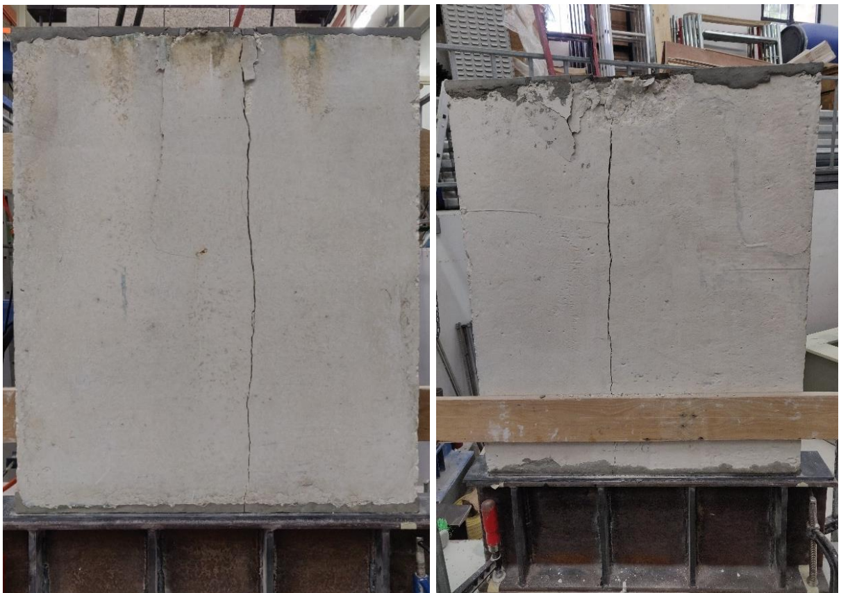
Figure 4.51 – Left , failure mode front elevation; right , failure mode back elevation
