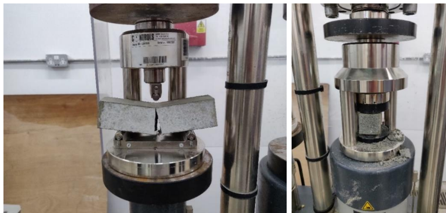
Figure E.1 – Testing grout sample in; left , flexure; right , compression
