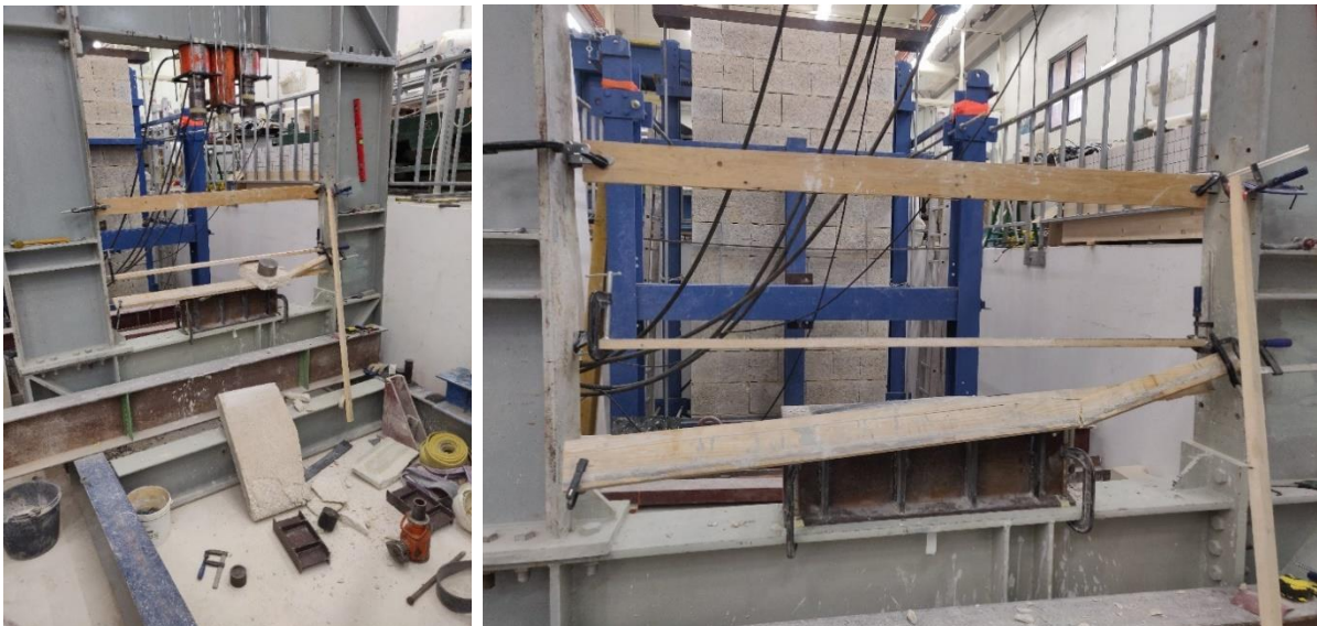
Figure 4.32 – Explosive wall failure
