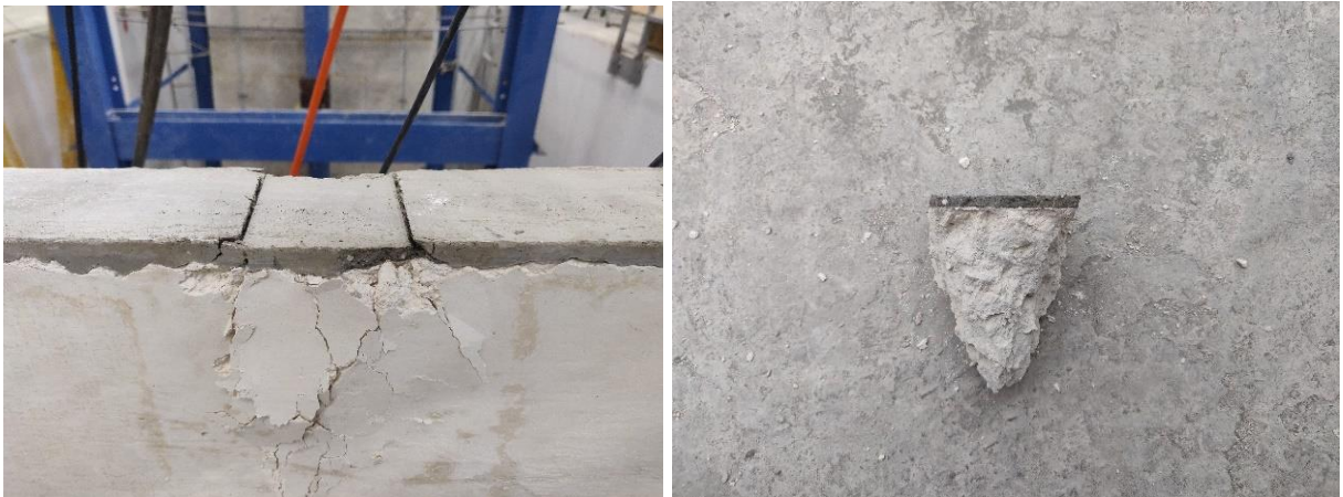
Figure F.22 – Failure mode wedge cone failure
