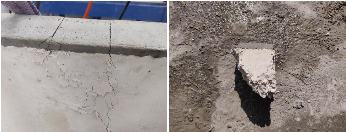
Figure F.18 – Failure mode wedge cone failure
