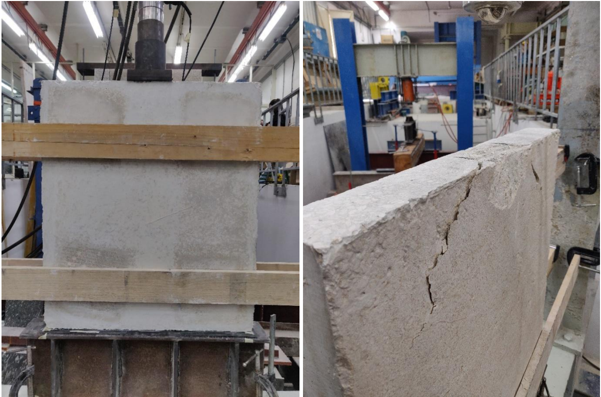
Figure F.32 – Left , front elevation showing no signs of failure; right , failure along the back elevation
