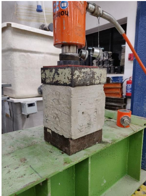
Figure D.1 – Prestressing the cube overnight using a Holmatro hydraulic loading jack
