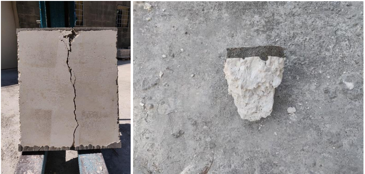
Figure F.20 – Left , failure mode front elevation; right , wedge cone failure
