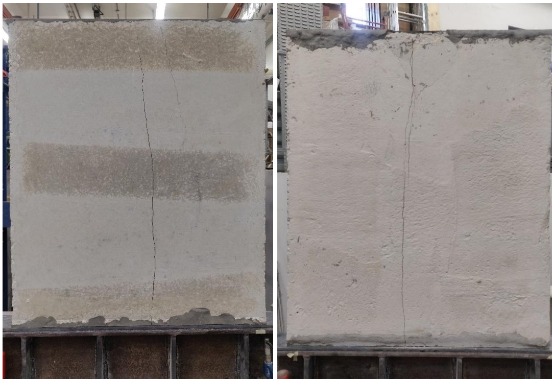
Figure 4.57 – Left , failure mode front elevation; right , failure mode back elevation
