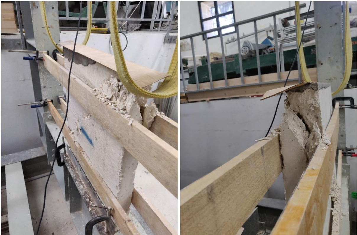
Figure F.6 – Left , failure mode back elevation; right , diagonal cracking failure through the top surface
