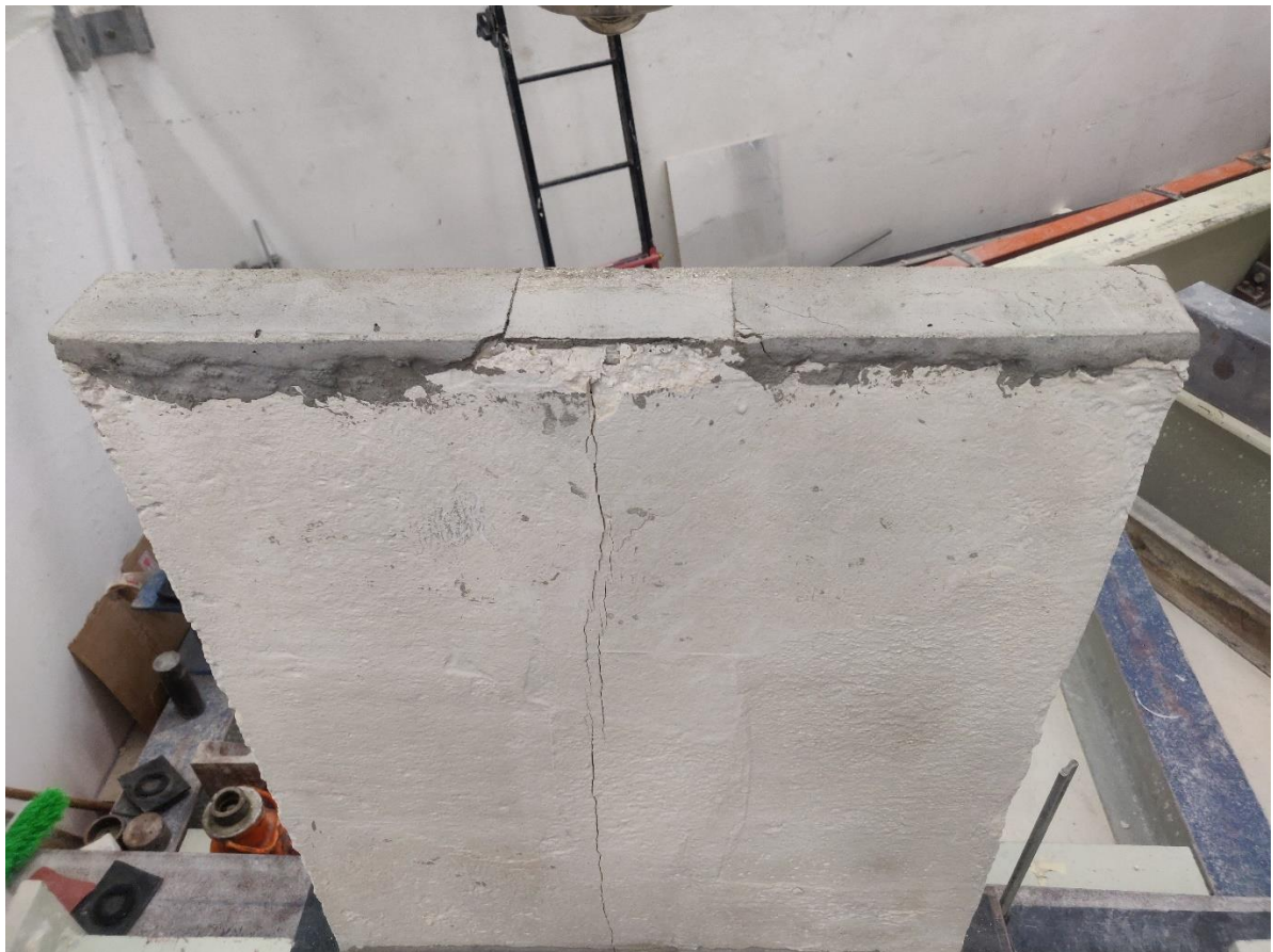
Figure F.49 – Concentrated load failure mode through the grout layer
