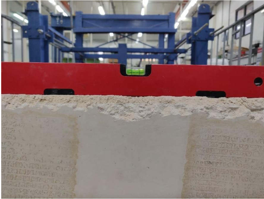
Figure F.3 – Using fine sands to level the loading surface
