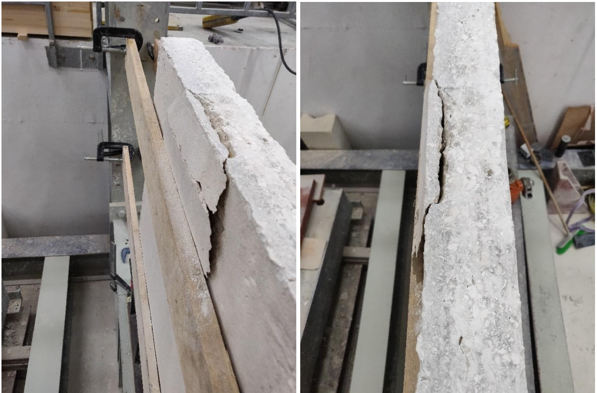
Figure F.35 – Failure along the back elevation; pressure along one particular side
