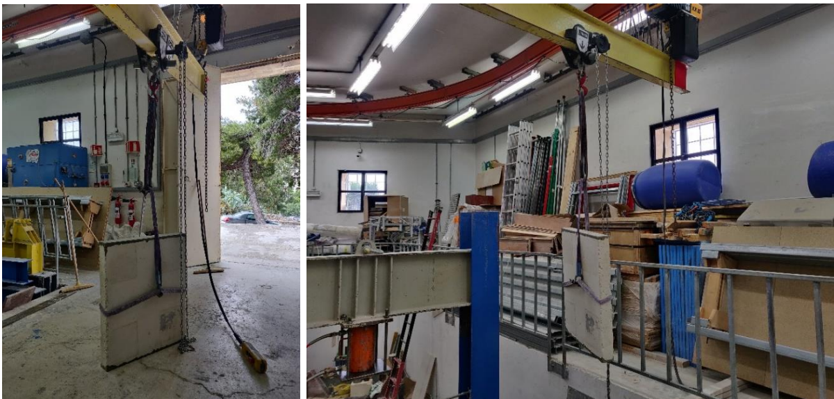
Figure 3.16 – Transportation of a typical wall within the lab using the overhead crane
