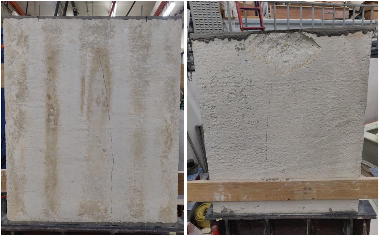
Figure 4.49 – Left , failure mode front elevation; right , failure mode back elevation
