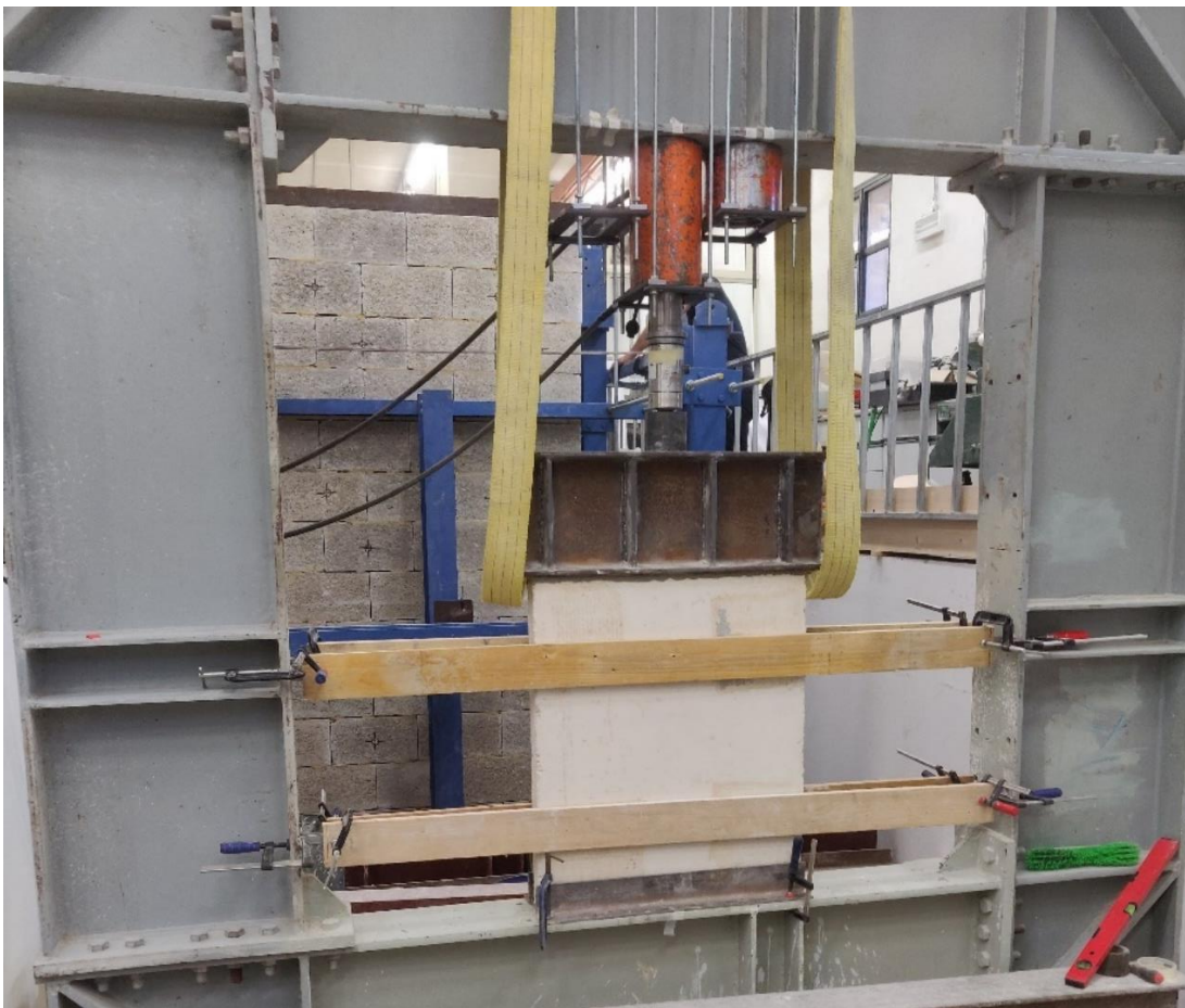
Figure 3.13 – Typical test performed with failure under UDL
