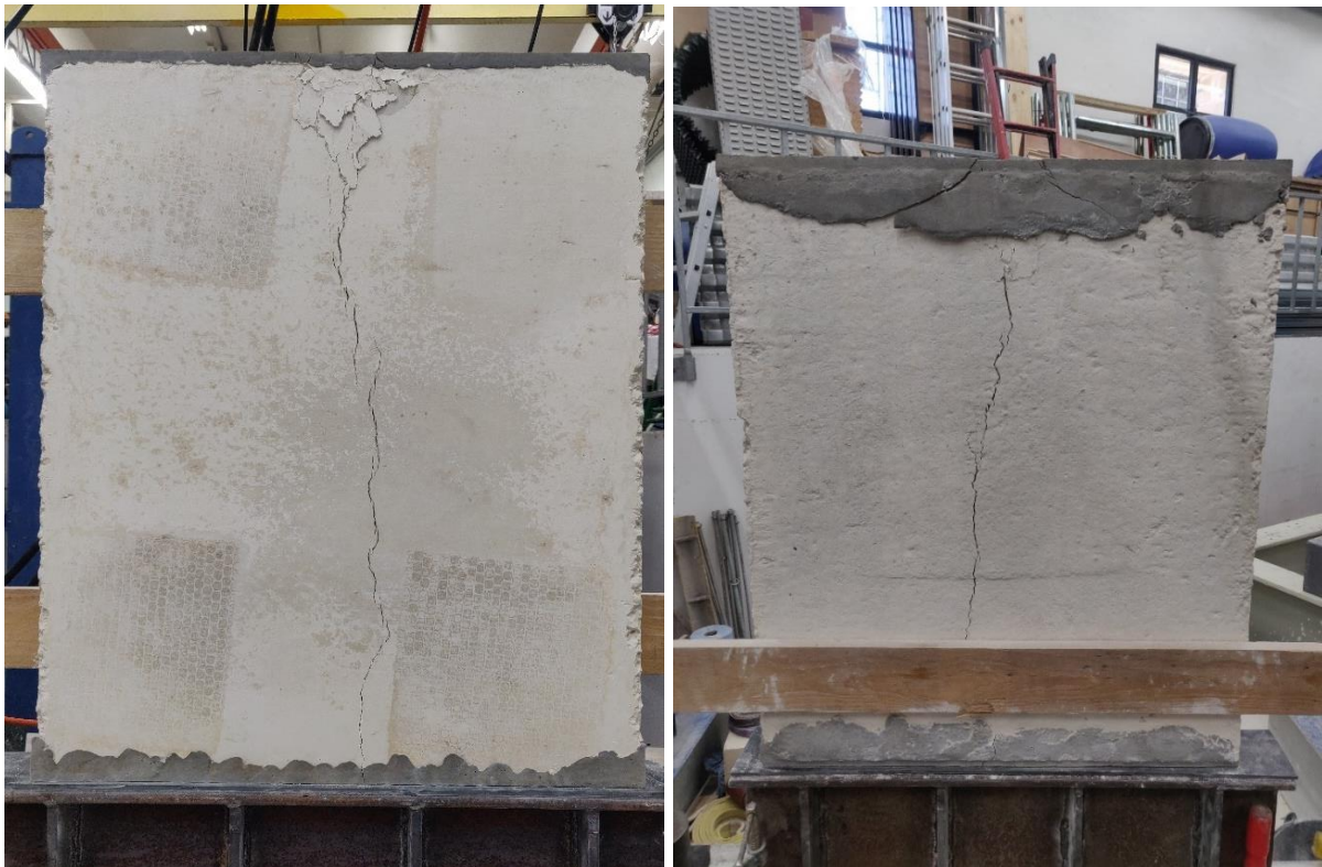
Figure 4.21 – Left , failure mode front elevation; right , failure mode back elevation
