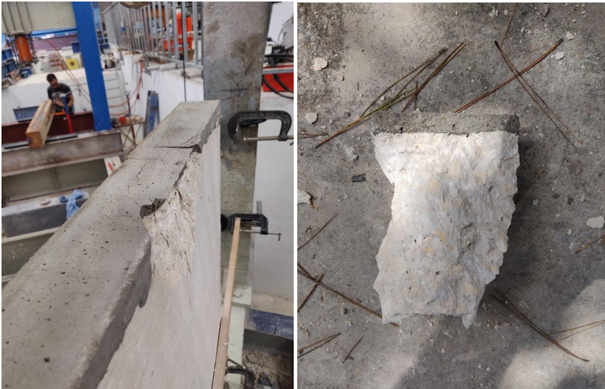
Figure F.45 – Concentrated load failure mode through the grout layer, forming a cone/wedge
