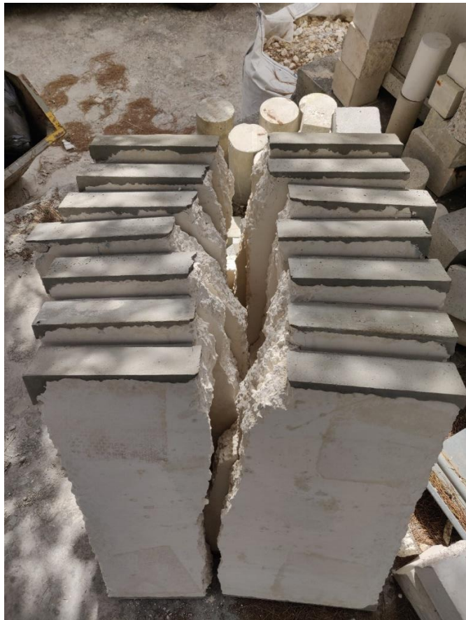
Figure G.5 – Majority of the wall panels post loading from the first testing programme
