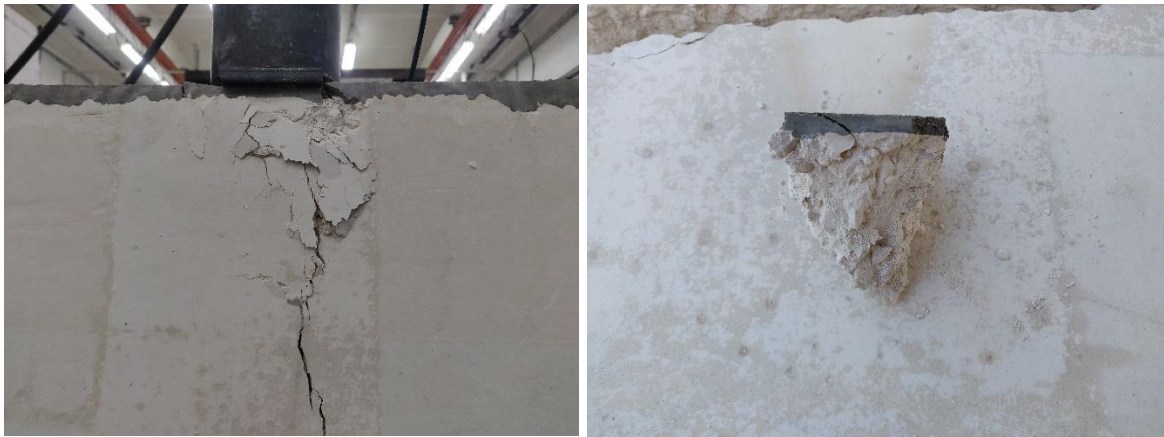
Figure F.10 – Wedge cone failure mode
