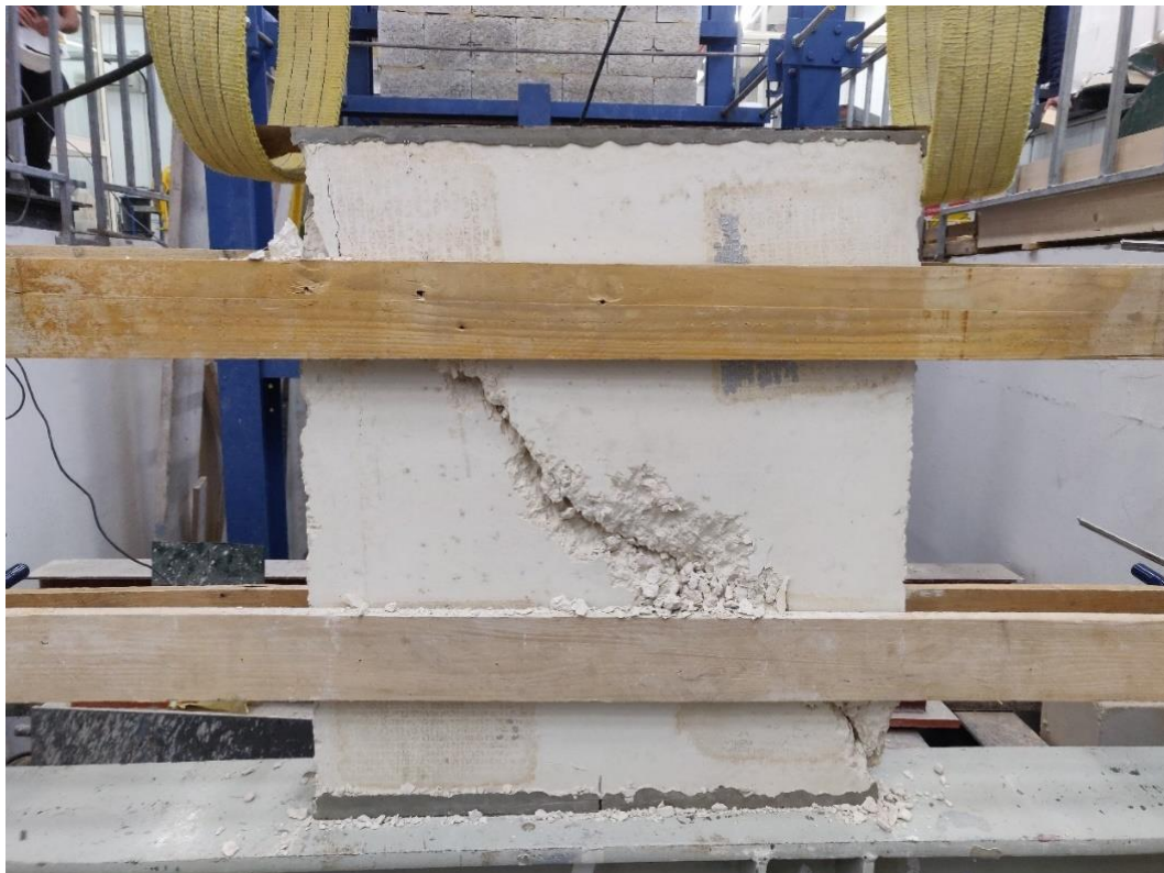
Figure 4.6 – Failure mode front elevation
