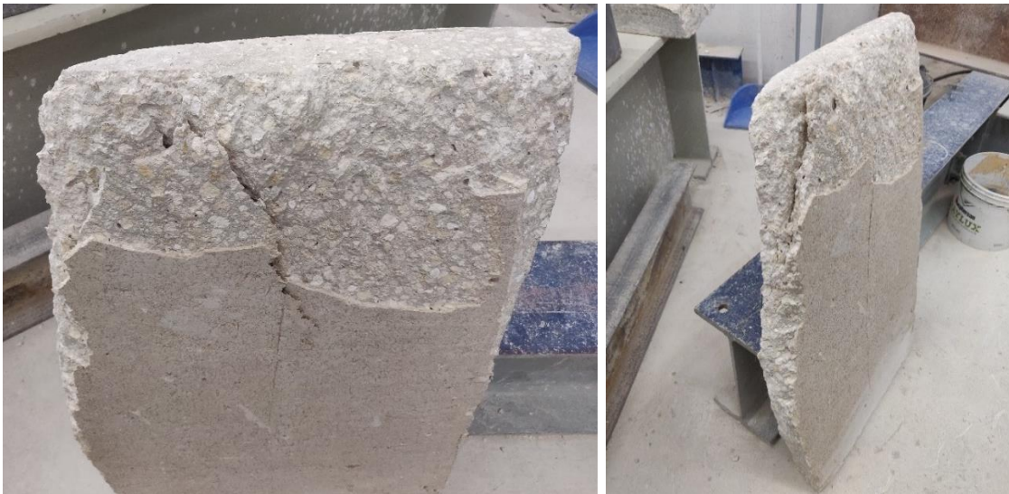
Figure F.28 – Failure mode under UDL loading
