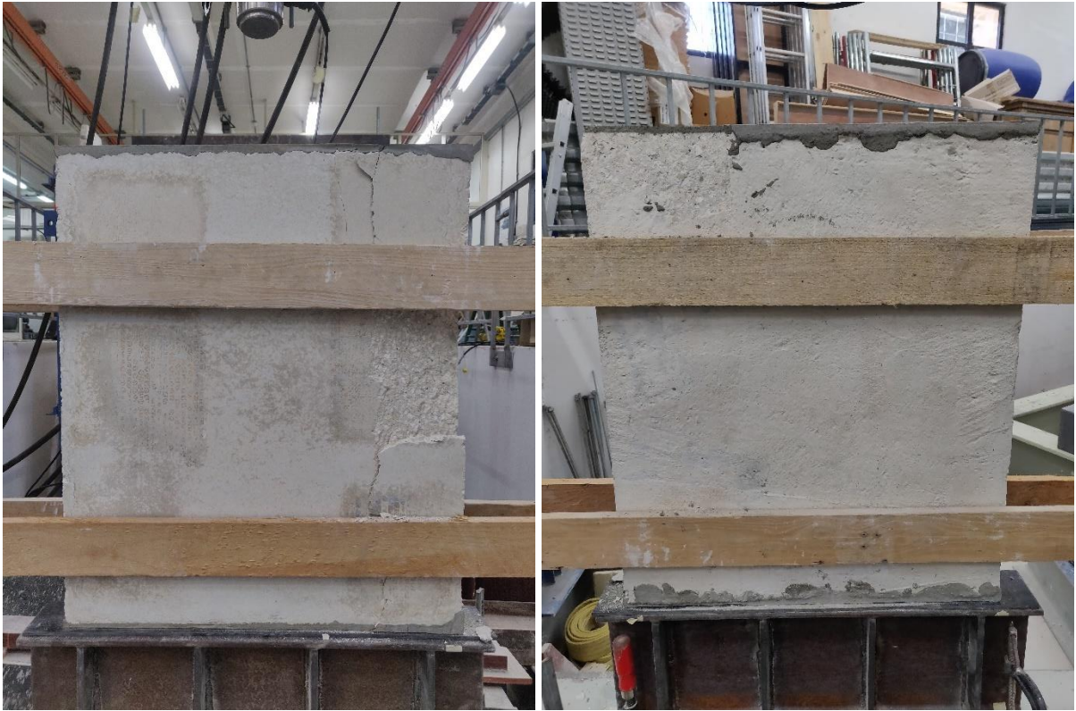
Figure 4.44 – Left , failure mode front elevation; right , failure mode back elevation
