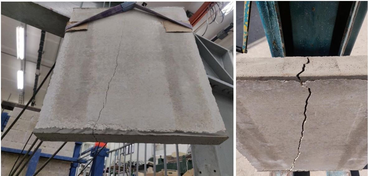
Figure F.39 – Failure through the grout layer
