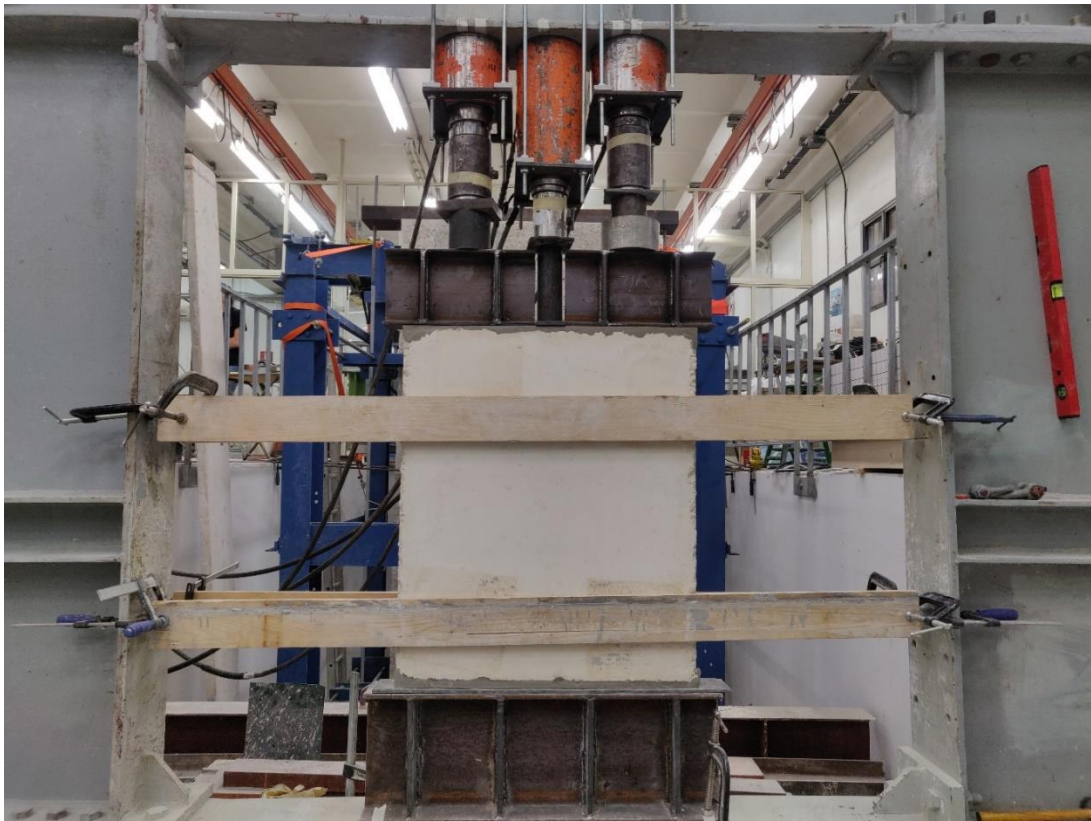
Figure 3.12 – Typical test performed, including both the precompression and concentrated loads
