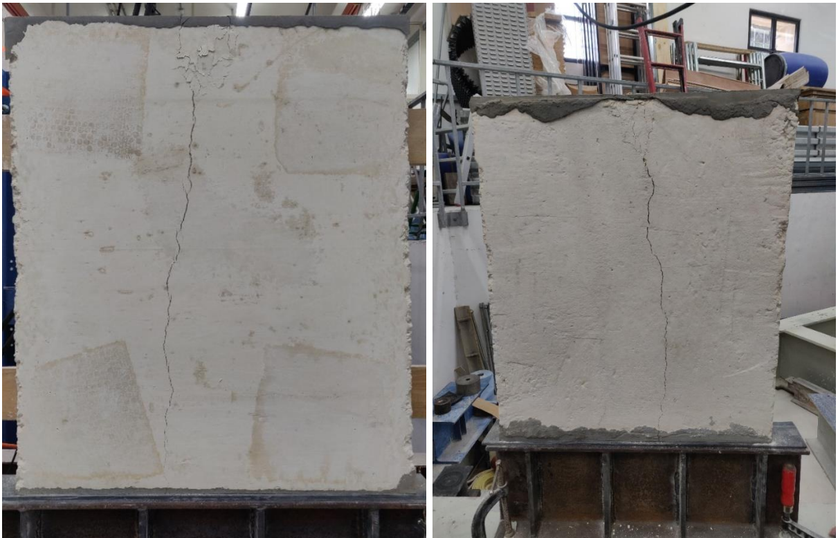
Figure 4.25 – Left , failure mode front elevation; right , failure mode back elevation
