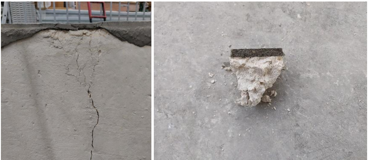
Figure F.24 – Failure mode wedge cone failure
