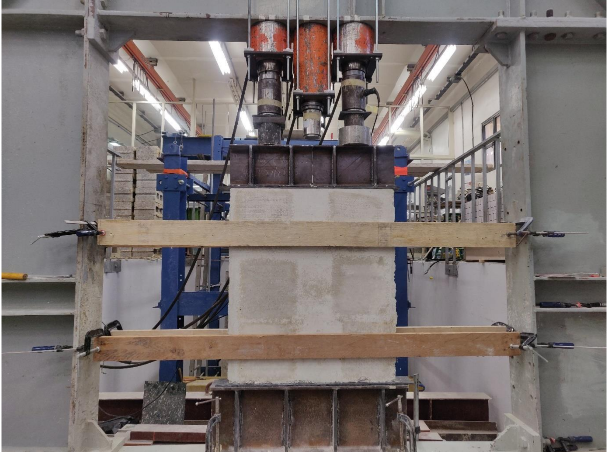
Figure 4.30 – UDL Loading setup for the second test programme
