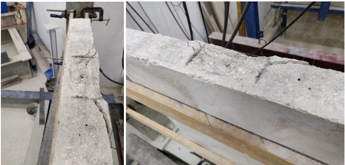
Figure F.33 – Concentrated load failure mode through the grout layer
