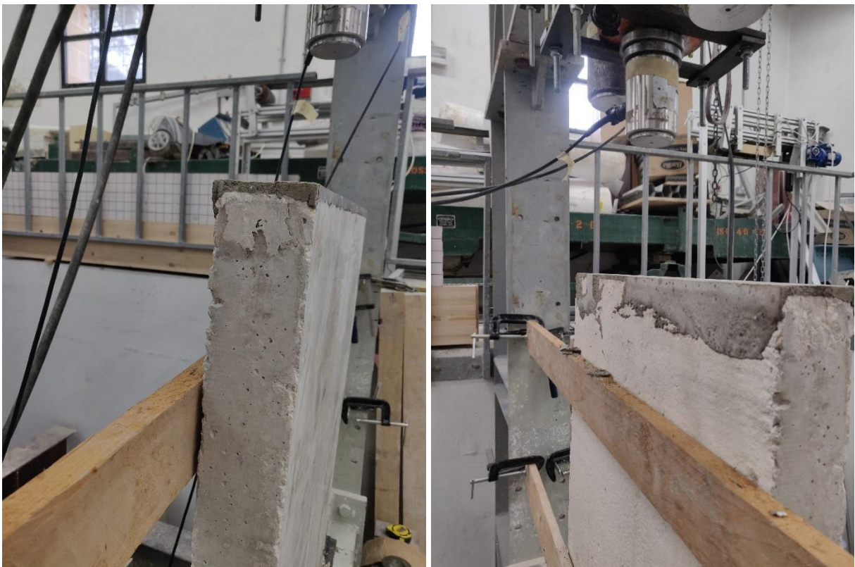
Figure 4.41 – Upper surface; brittle spalling of the concrete and grout layer
