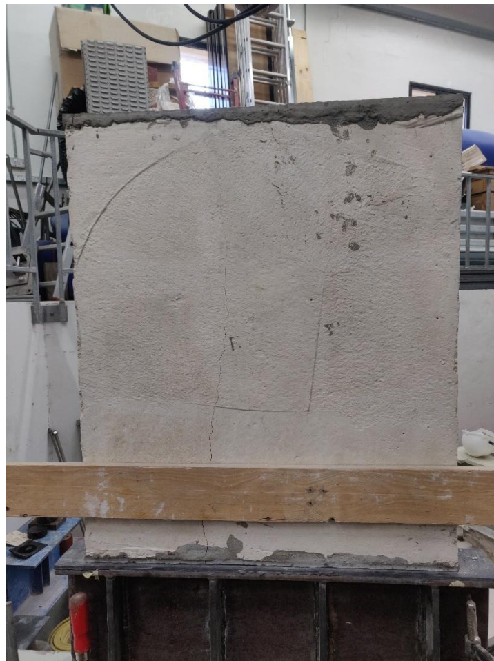
Figure F.47 – Failure mode back elevation
