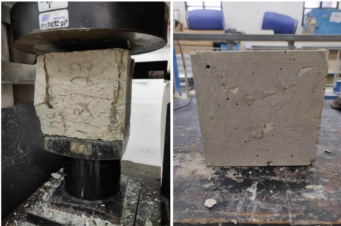
Figure D.2 – UCS cube failure mode for; Left , cube 3; right , cube 4
