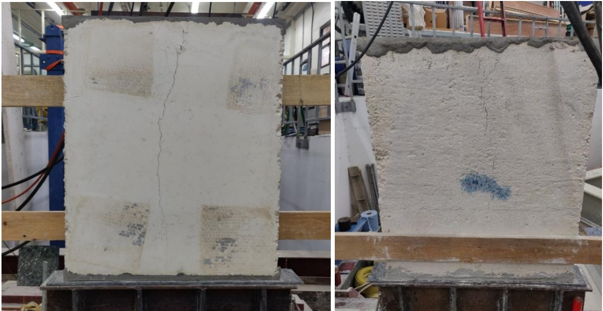
Figure 4.13 – Left , failure mode front elevation; right , failure mode back elevation
