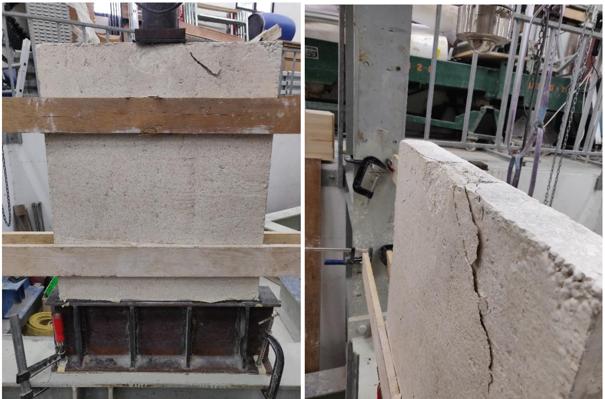
Figure 4.36 – Failure mode back elevation
