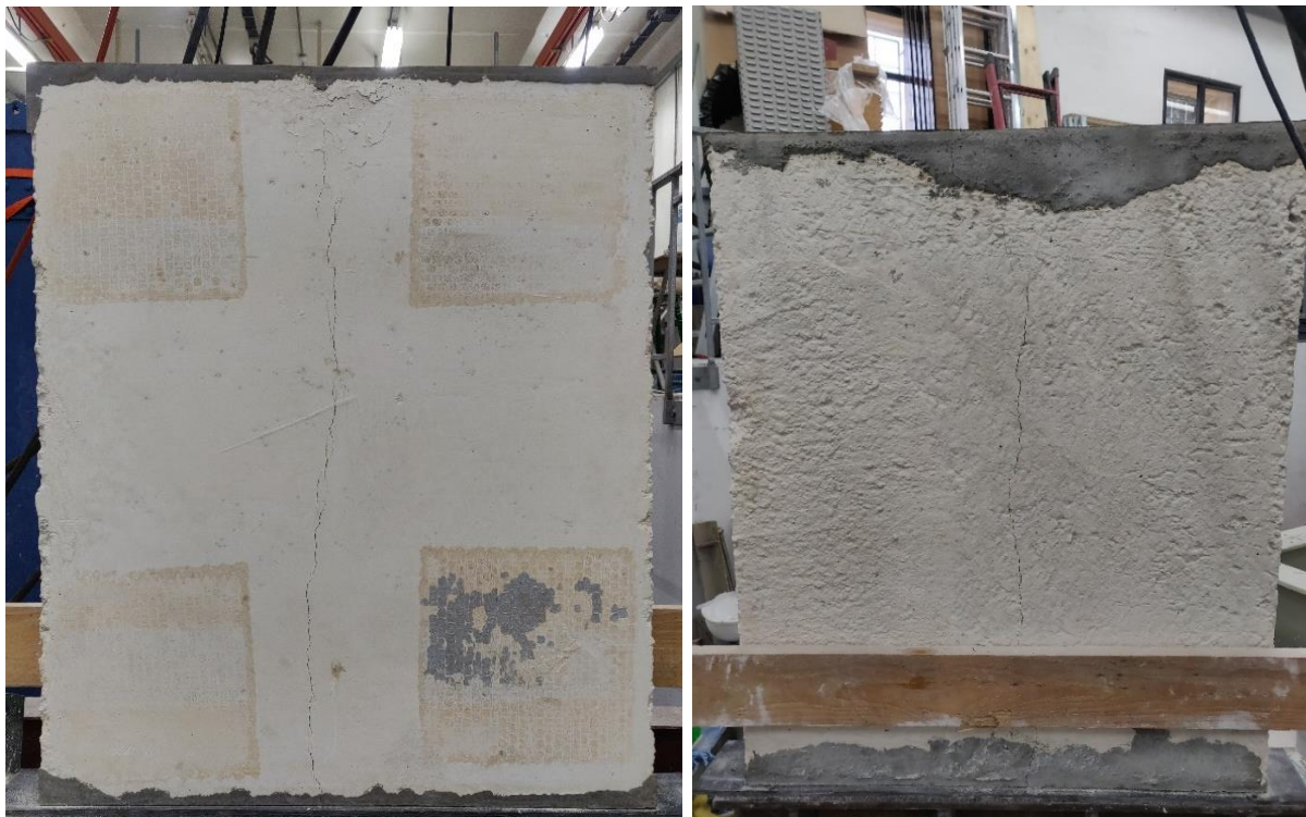
Figure 4.15 – Left , failure mode front elevation; right , failure mode back elevation
