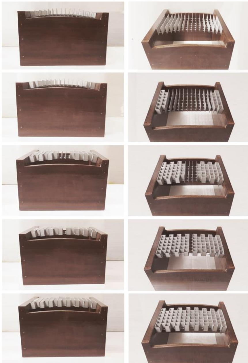
Figure 3.27: The construction of a shallow segmental vault with a rise to span ratio of 0.033 Left: Elevation of the erection process; Right: Planar view of the erection process
