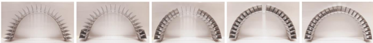
Figure 3.13: The construction of a 3D printed semicircular arch
