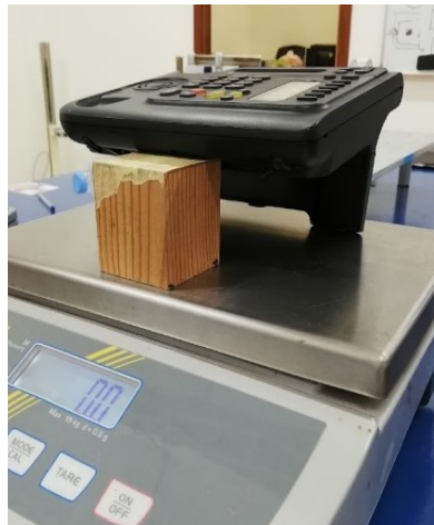
Figure C.8: The set-up used to measure the force applied on the telephone when dialling a number.
