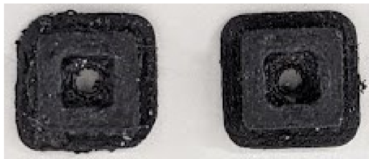
Figure H.2: The observed deformation in the interface keys mounted on the Index MCP shaft
