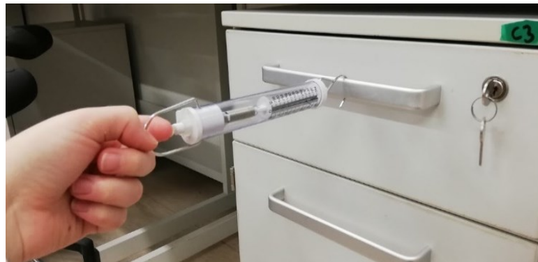
Figure C.7: The set-up used to determine the force required to open a drawer
