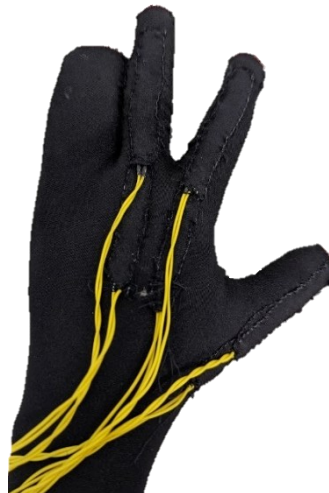
Figure 4.14: The developed data glove equipped with six 2-inch RFSs
