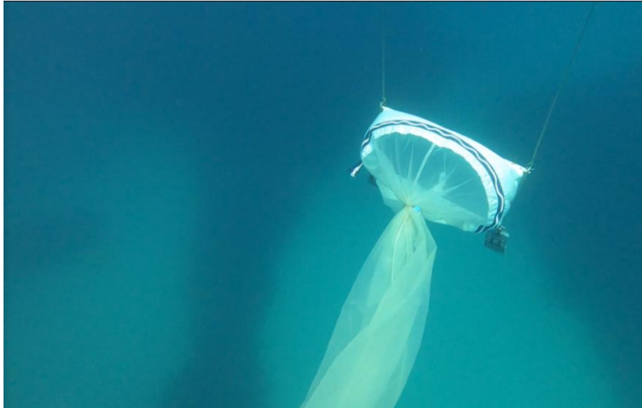
Figure 14 Closed manta-net prior the commencement of the sampling.
