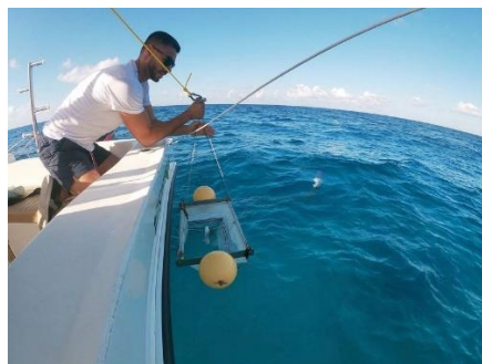
Figure 11 Removing Manta-net from the sea after sampling
