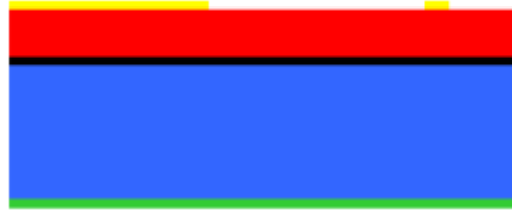
Figure A.1 ~ Thermal oxide layer shown in yellow over the silicon layer.
