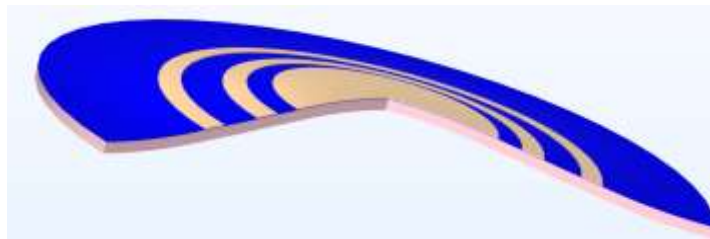
Figure 3.26 ~ Multiple electrode PMUT showing the electrodes on top in aluminium colour, the AlN layer in blue underneath and the pink silicon diaphragm.
