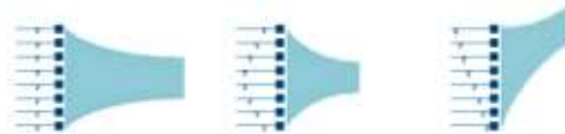
Figure K.6 ~ A schematic which shows the principles of ultrasonic beam steering and focusing in an array system [100].
