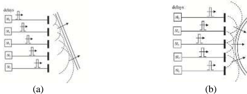
Figure K.5 ~ Beam being steered through specific delays introduced in the signal to each of the transmitters [155].
