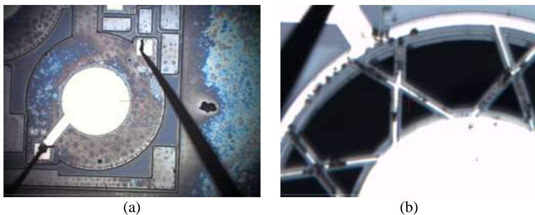
Figure 5.4 ~ Damage effects to (a) piezoelectric and (b) pad metal layers due to the combination of ultrasonic radiation and water.
