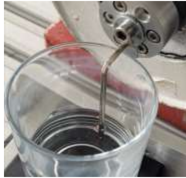
Figure Q.1 ~ Concept of the frequency adjustment procedure showing source of vibration at the top right hand corner with metal vibrating laser target in the fluid test container.
