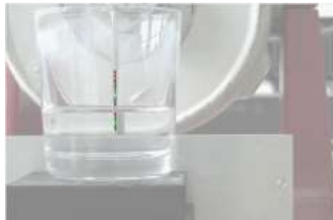
Figure Q.2 ~ Side view showing the metal vibrating laser target partially in liquid and partially in air.
