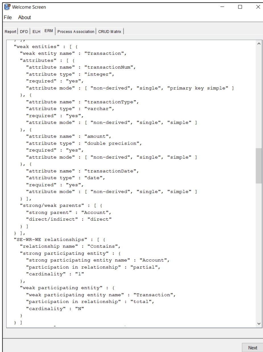
Figure 7.2: JSON-formatted ERM snippet representing a 'Banking' system
