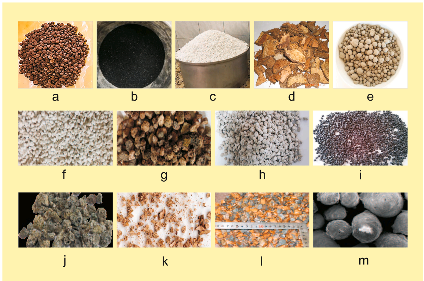
Figure 2. The shape of different types of LWA: a. expanded clay (Nahhab and Ketab, 2020); b. rubber (Hossain et al., 2020); c. EPS (Medher et al., 2021); d. coconut shell (Poongodi and Murthi, 2020); e. fly ash aggregate (Güneyisi et al., 2016); f. perlite (Dolatatabad et al., 2020); g. scoria (Dolatatabad et al., 2020); h. pumice (Agwa et al., 2020); i. recycled plastics (Faraj et al., 2021); j. POC (Feen et al., 2017); k. olive kernel shells (Cheboub et al., 2020); l. expanded shale (Wu et al., 2009); m. expanded glass (Spiesz et al., 2013).
