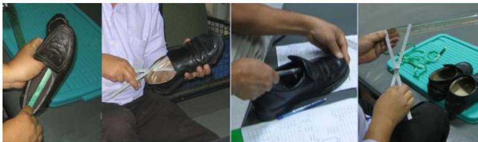
Figure 2.7. Using tape measure ( 1 st picture on left) and shoe callipers to measure footwear internal length and width (Chaiwanichsiri, Tantisiriwat, & Jachai, 2008).
