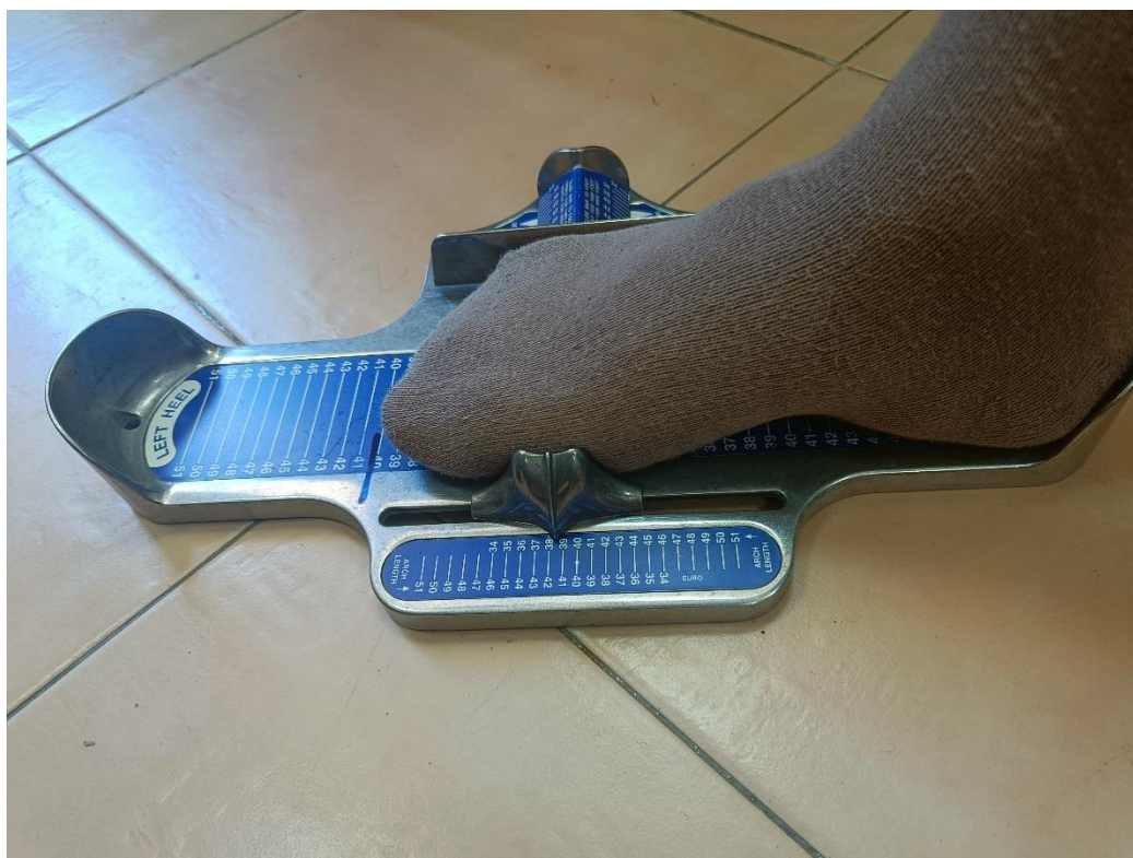
Figure 3.2 Measuring footwear length using the Brannock Device
