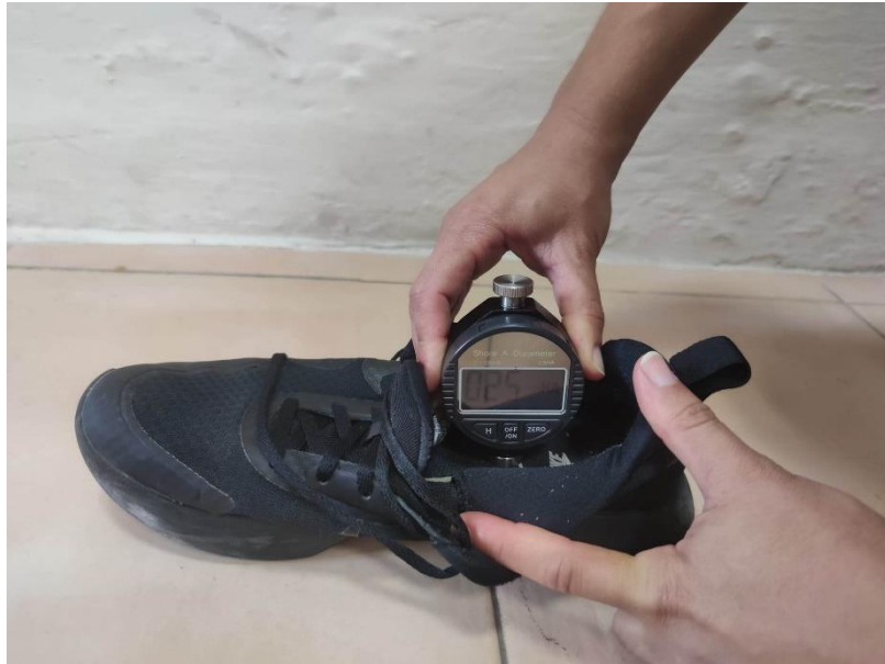
Figure 3.1 Using the shore A durometer to measure sole hardness.
