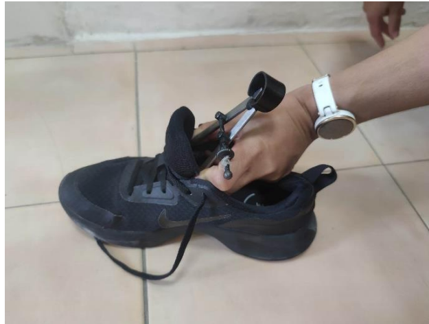
Figure 3.7 Using the spring calliper to measure the internal width of the shoe.
