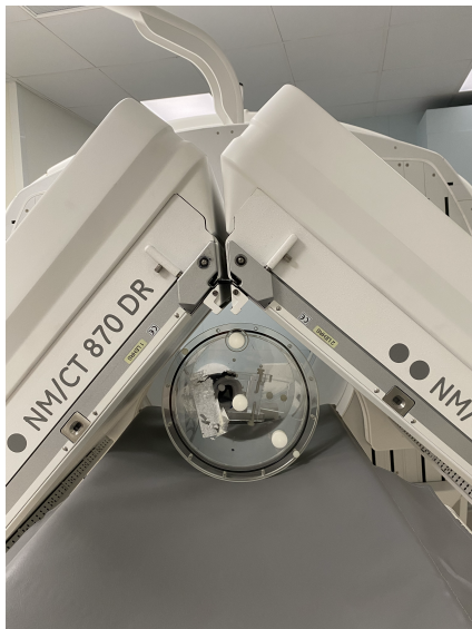
Figure 3.3: 3D-printed phantom in NM/CT 870 DR
