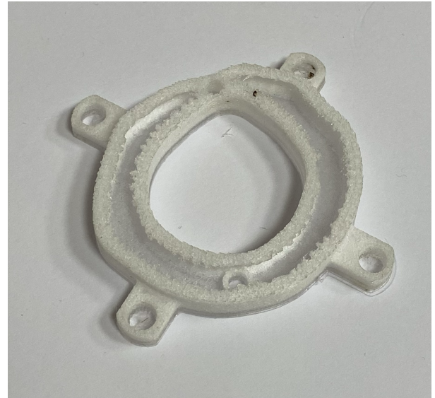
Figure 3.10: Ultimaker - failed print because of bad extruder
