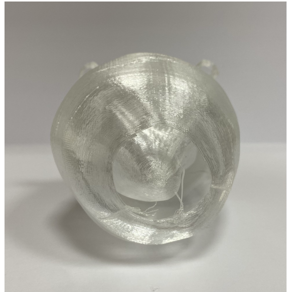
Figure 3.8: Failed overhang to enclose phantom at the apex of the heart
