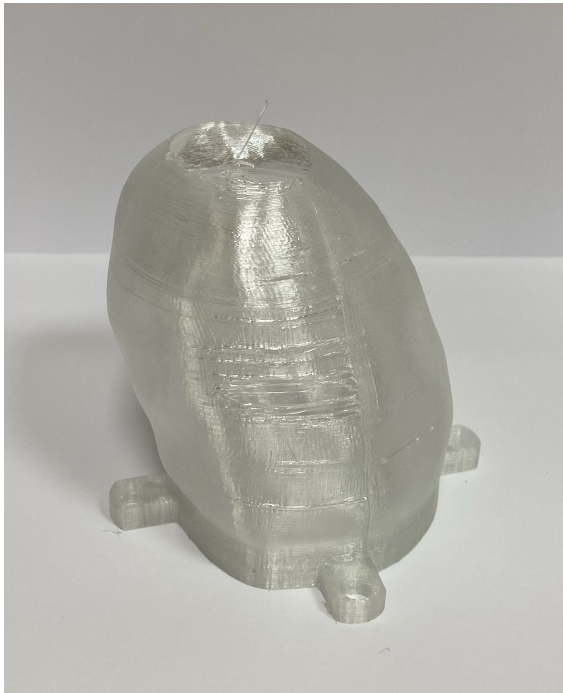
Figure 3.7: Hole and inconsistencies in the sides of the phantom
