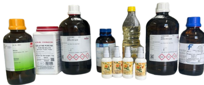
Figure 3.3: Ingredients used in the fabrication of the oil-in gelatin phantoms. From left to right: Kerosene oil, 200 Bloom Gelatin, deionised water (two separate bottles), p-toluic acid, sunflower oil (back), safflower oils (front), Propan-1-ol.
