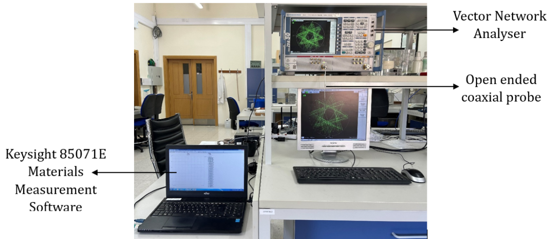
Figure 3.1: Setup of the VNA, probe and the software used
