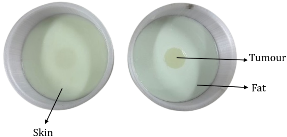
Figure 4.4: Oil-in-gelatin phantoms: from left to right—phantom with the skin mimic and phantom without the skin mimic
