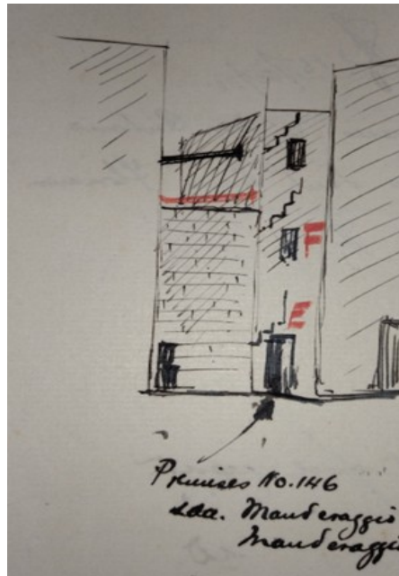
Fig. 58. Sketch of primary remedial works on a dangerous structure at No. 146 Strada Manderaggio , Valletta. 78
