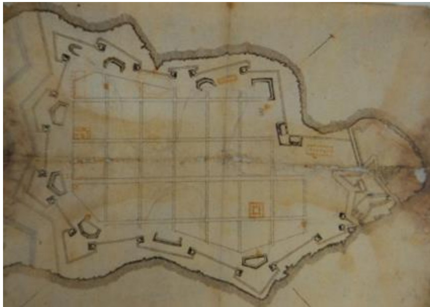
Fig. 7. The plan by Laparelli in which he introduced the iron-grid street pattern. (Denis de Lucca)
