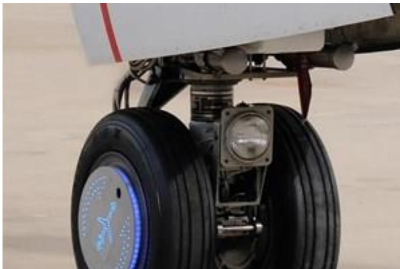
Fig. 2. WheelTug technological solution [28].
