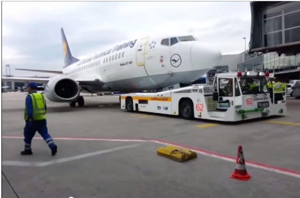
Fig. 3. TaxiBot system in operation at Frankfurt airport [34].
