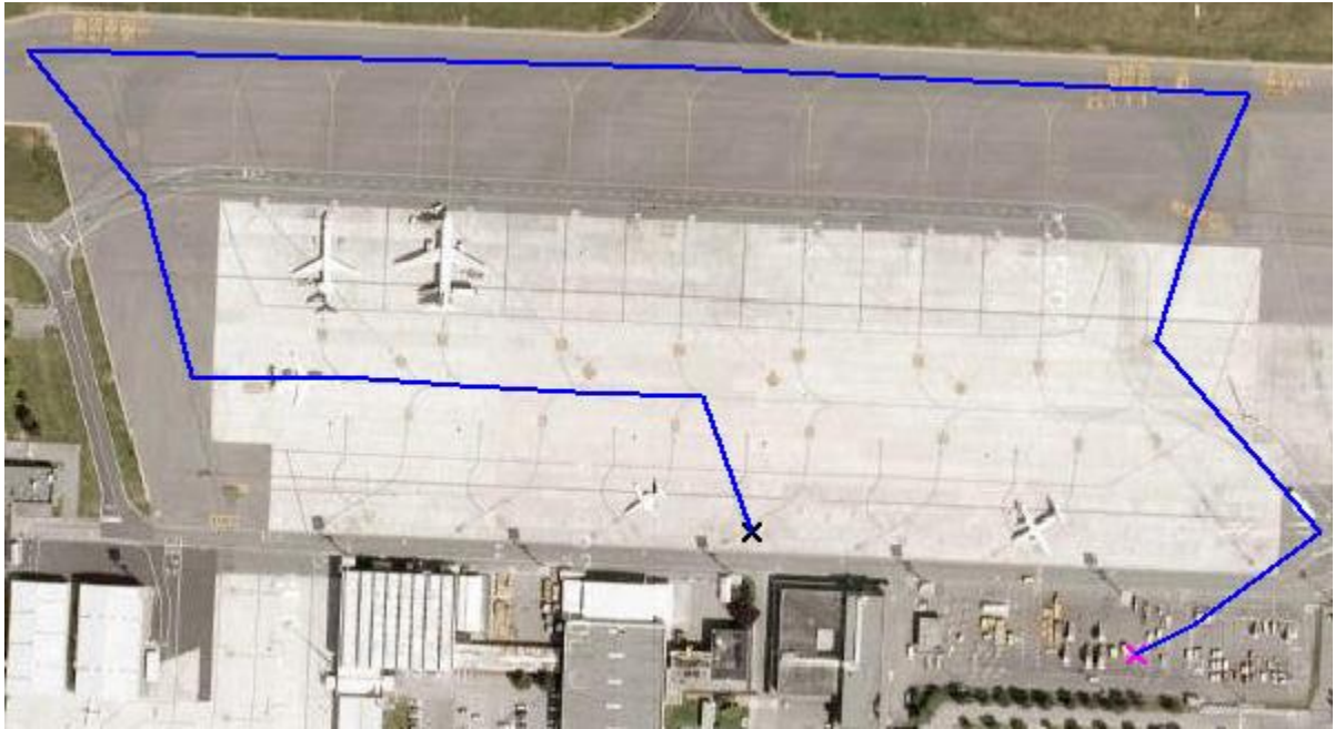
Fig. 6. Example of a tow truck route in Sandro Pertini Airport of Turin from a tow truck depot to a departing aircraft. This route was calculated using the standard HNN algorithm [48].
