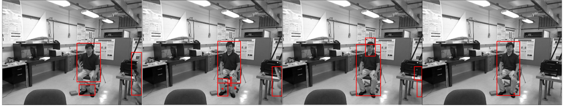
Figure 4.6 Visual results using motion saliency showing multiple regions identified that pertain to the same object
