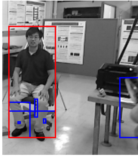
Figure 4.9 Example of bounding rectangle (red) covering union box of regions (blue) that overlap with Kalman filter window
