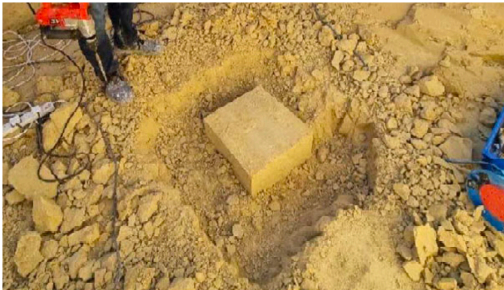
Figure 4.8 - Trial pit dug in the Upper Globigerina Limestone (Falzon, 2022)
