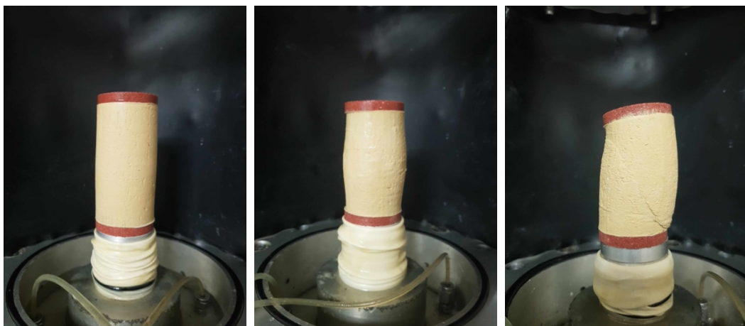
Figure 5.10 – Failure mode of the Reconstituted R1_U_200 (Left), R2_U_400 (Middle) & R3_U_800 (Right)
