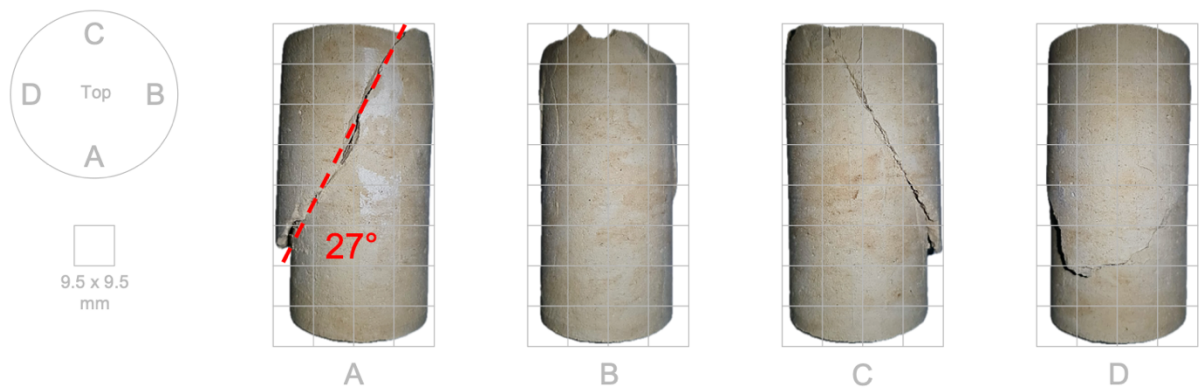
Figure 5.22 - Photos representing the failure mode of specimen N1_U_200 from four different angles
