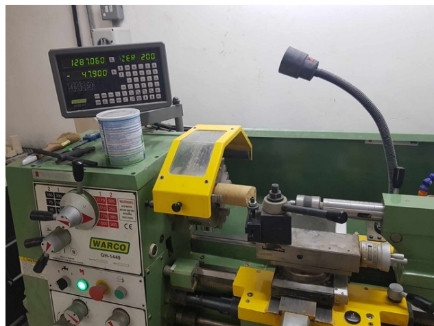
Figure 4.11 - Lathe machine tool used to trim the natural UGL-2 sample to size
