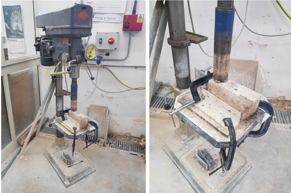
Figure 4.10 - Pillar drilling of natural Upper Globigerina Limestone
