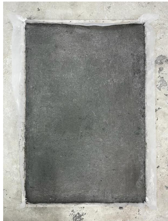
M0.5S Mix – No Cracks
