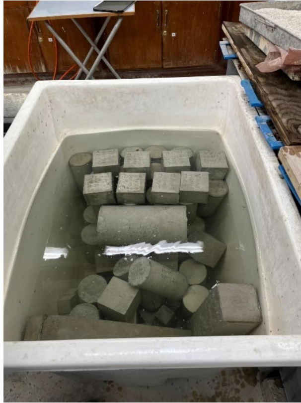
Figure 3.15 - Specimens curing in Controlled Water Tank (BS EN 12390-2:2009, 2009).
