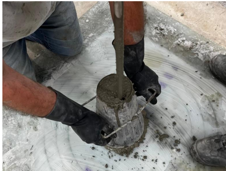
Figure 4.15 - Slump Cone being tamped for 25 times.
