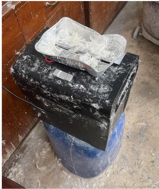
Figure 4.8 - Modified Paper Shredder used to Trim Feather Fibres to a Shorter Length Range.
