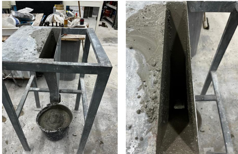
Figure 4.17 - Viscosity - V-Funnel test apparatus after use.
