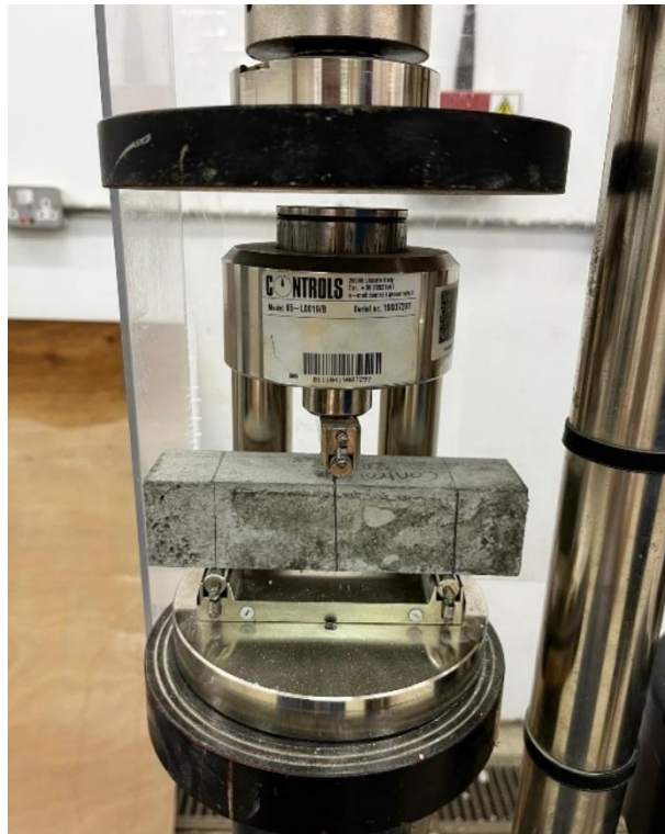
Figure 3.23 - Mortar Flexural Test Setup (BS EN 1015-11:1999, 1999).
