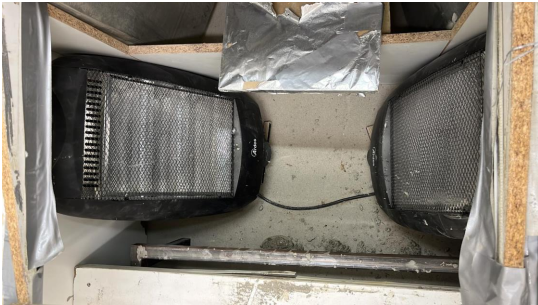
Figure 3.34 - Halogen Heaters inside the Environmental Chamber.
