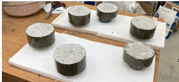
Figure 3.39 - Specimens while outer Epoxy Resin Coating is Curing (ASTM C1202-12, 2012).
