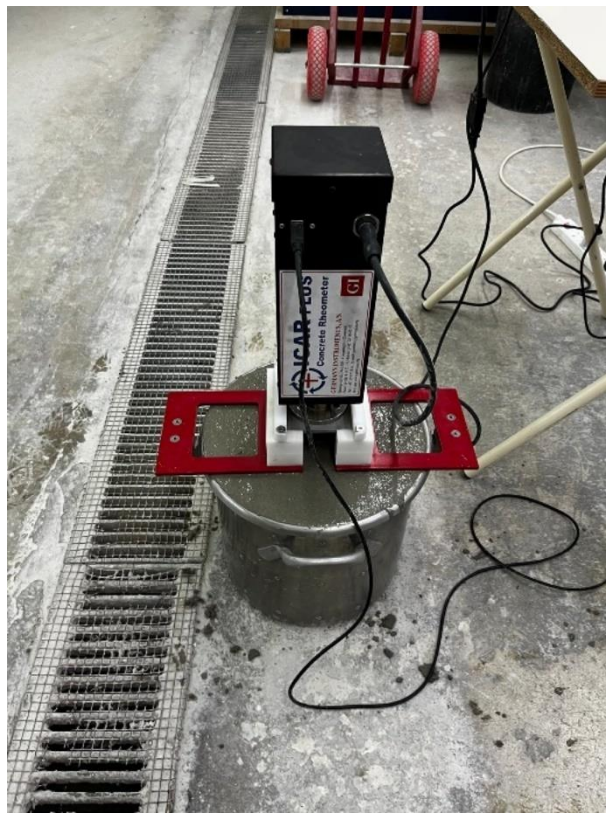
Figure 3.19 - ICAR Plus Concrete Rheometer.
