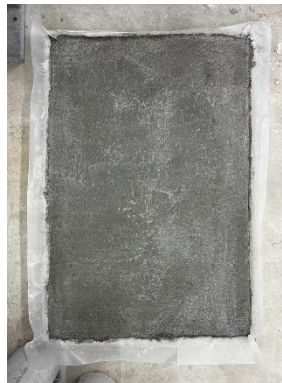
M0.25S – No Crack Formed
