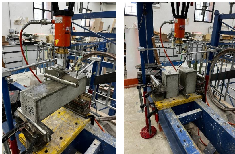
Figure 4.37 – Flexural Strength Test before and after Failure.
