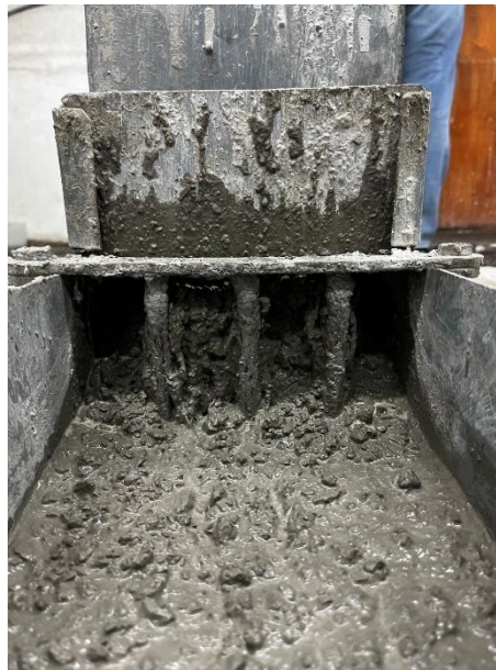
Figure 4.20 - Passing Ability - Fibres Clogging in L-Box Test showing reduced Passing Ability.
