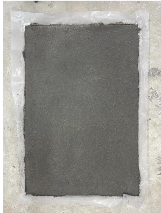
M0.125S Mix – No Cracks
