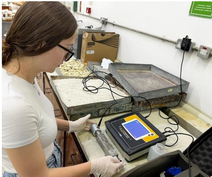
Figure 4.26 - Ultrasonic Pulse Velocity of a prism being measured.
