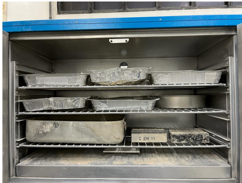
Figure 3.9 - Oven used for Drying Fibres at 50°C for 24 hours.
