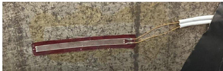
Figure 3.31 - Strain Gauge attached to the inner wall of the Ring.
