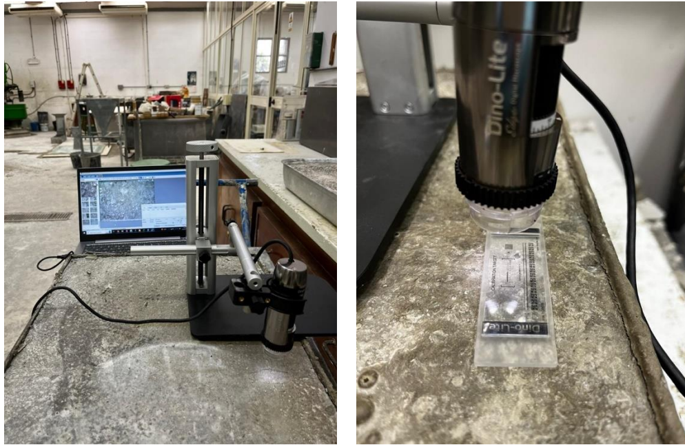
Figure 3.37 – USB Microscope used to Measure Cracks after 24 hours.
