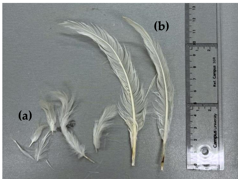
Figure 3.12 - The long, stiff feathers (b) were removed. The separation was done manually in order to leave only short, flexible fibres (a) for shredding.
