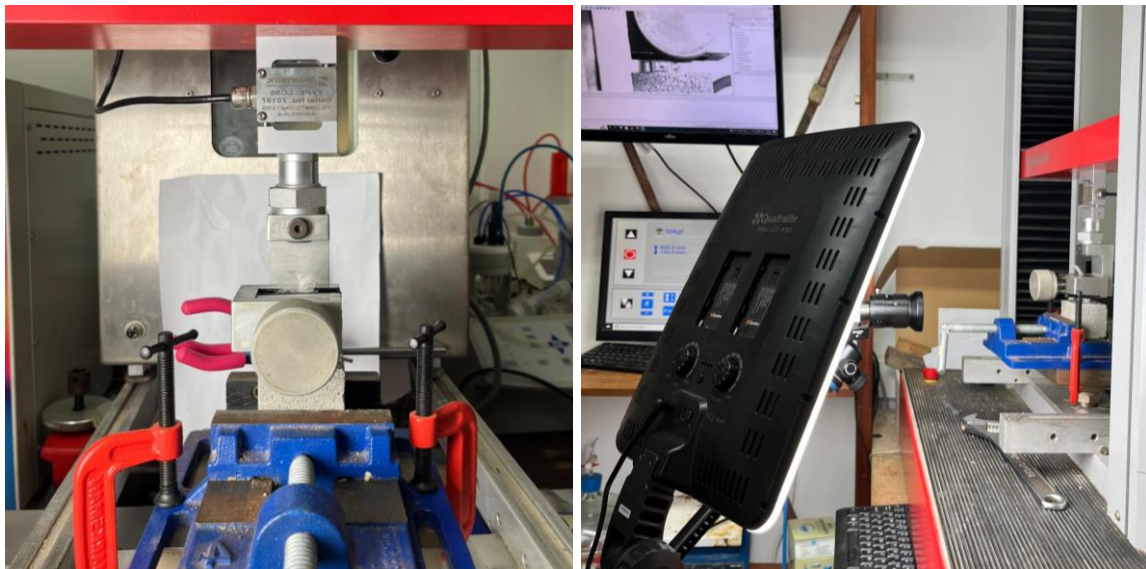
Figure 3.29 - Sample set up in Tensile Loading Machine with 500 N load cell (left) and Camera (right).
