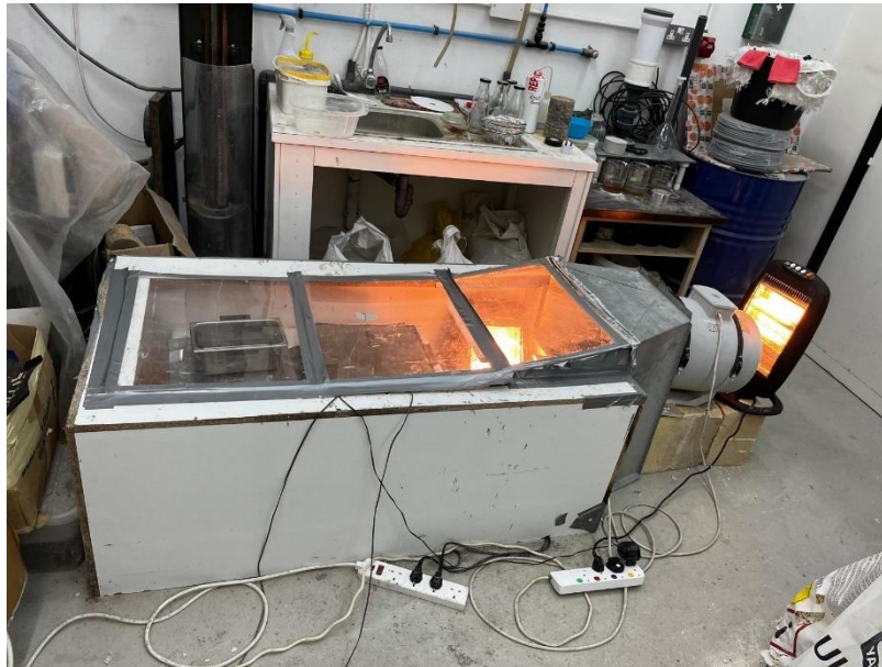
Figure 3.33 - Environmental Chamber Setup adapted chamber (ASTM C1579-06, 2006).
