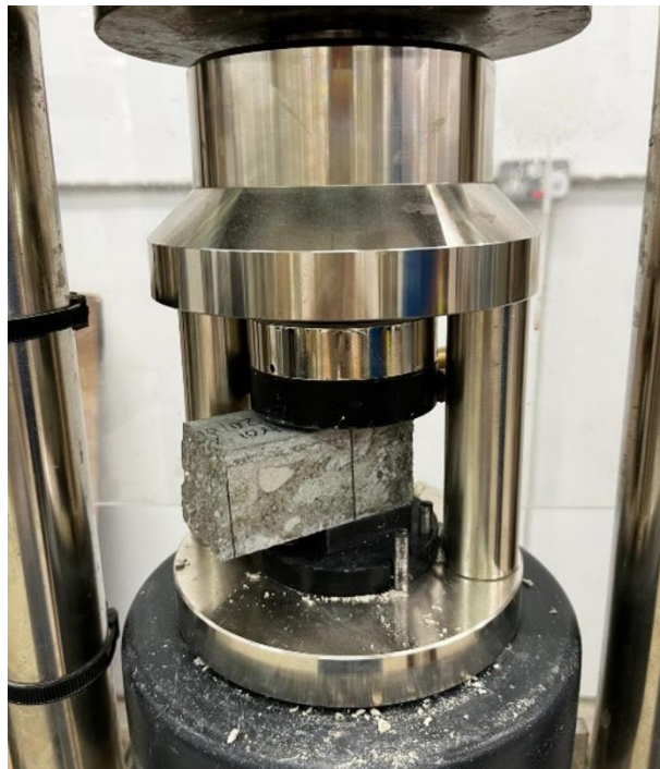
Figure 3.24 - Compression Test Setup (BS EN 1015-11:1999, 1999).
