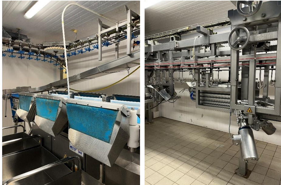
Figure 10 - (right) Conveyer belt which sorts the chicken by weight into four bins (left) Machine which cuts the chicken into parts by order.
