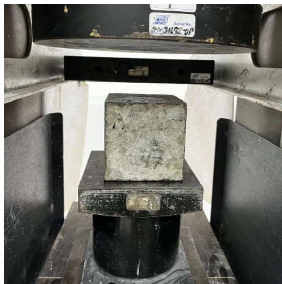
Figure 3.25 - Concrete Cube Compression Test Setup (BS EN 12390-3:2009, 2009).
