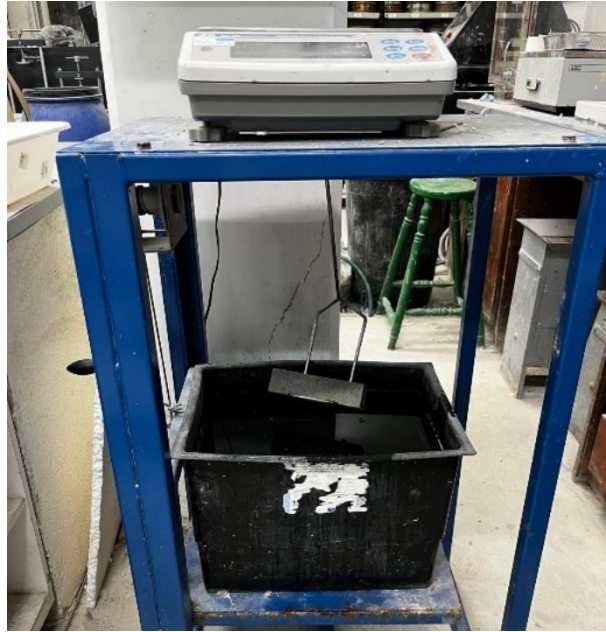
Figure 3.21 - Mortar Prism on the Stirrup before Submersion (BS EN 12390-7:2009, 2009).
