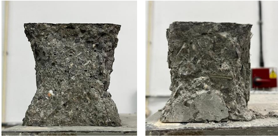
Figure 4.33 – Compressive Test Cubes after Failure – Fibres visible in some faces.
