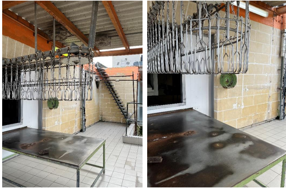
Figure 3 - Chain where chickens are hung upside-down to enter the plant.
