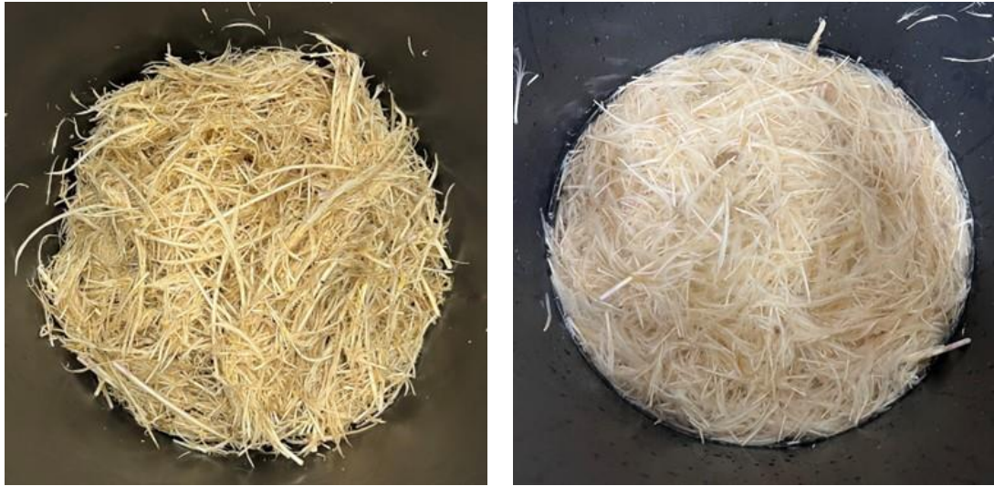
Figure 3.7 – Feather Fibres before (left) and after (right) Cleaning Process.
