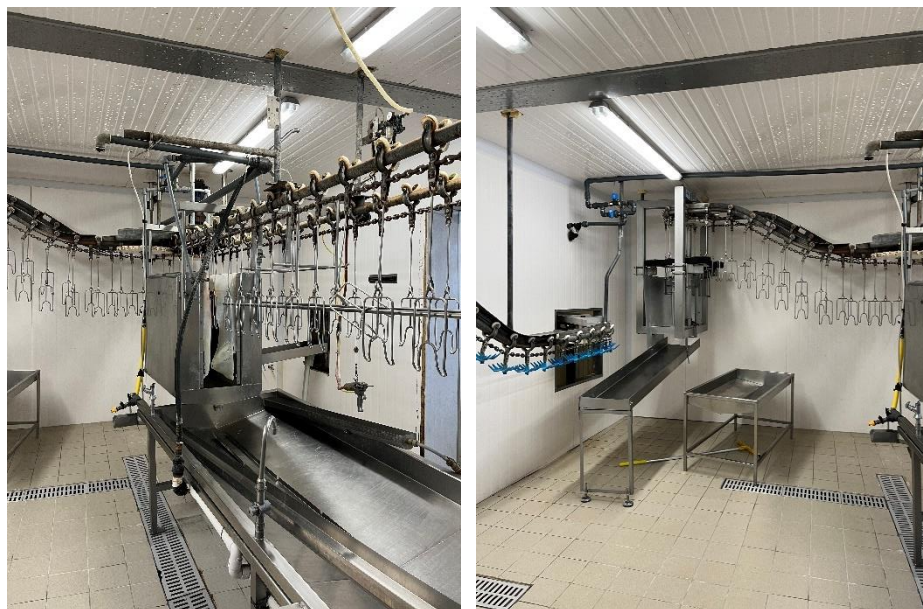
Figure 8 - Removal of internal organs, mostly manually operated.
