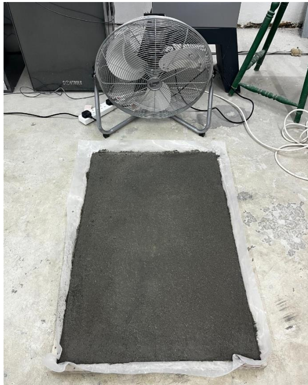
Figure 4.53 - Kraai Test after 6-hour Wind Loading Period.
