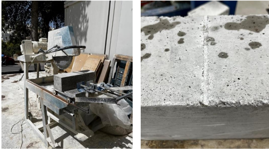
Figure 3.27 – Table Saw and 5mm Ridge cut in Flexural Test Specimens (BS EN 14651:2007, 2007).
