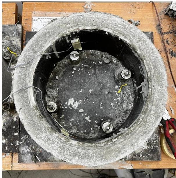
Figure 3.32 - Top View of Ring Specimen during the 28-day testing duration.
