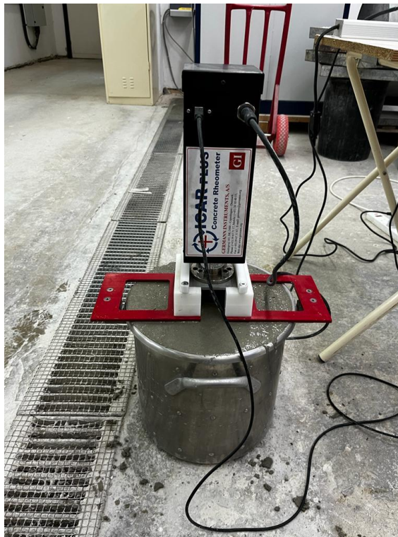
Figure 4.22 - ICAR Plus Concrete Rheometer in use.
