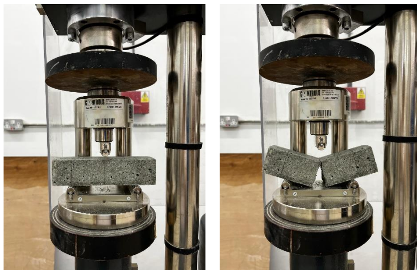
Figure 4.28 – Mortar Prism before and after Failure in the Three-Point Bending Test.
