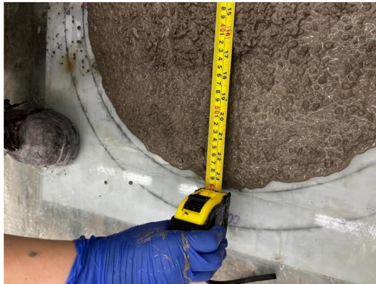
Figure 4.12 - Slump flow diameter being measured.
