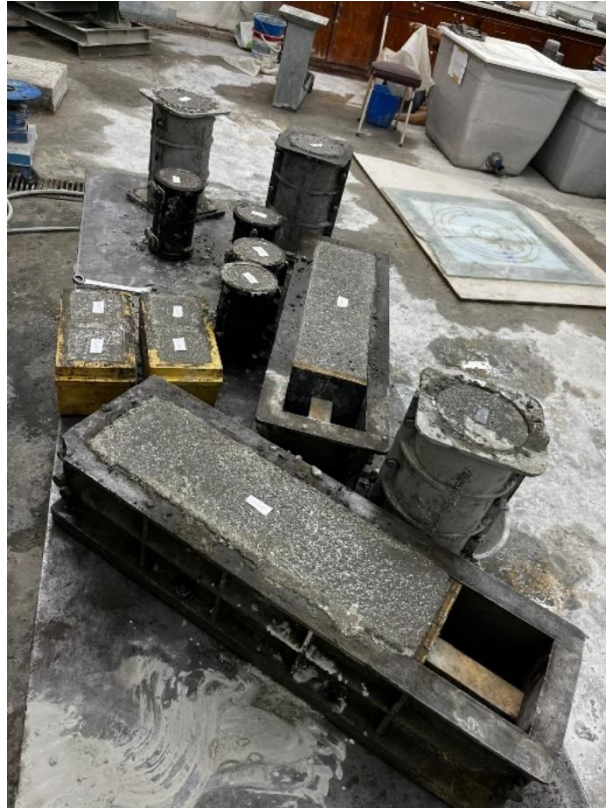
Figure 3.14 - Samples cast in the various Moulds to be Demoulded.
