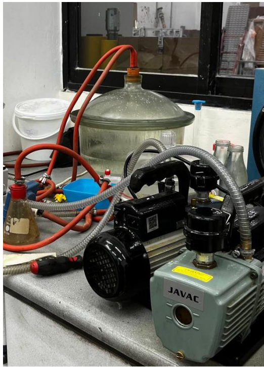
Figure 3.40 - Conditioning Setup for Chloride Penetration Samples (ASTM C1202-12, 2012).
