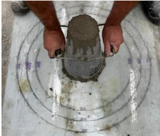
Figure 3.16 - Slump Flow Test Setup (BS EN 12350-7:2009, 2019).
