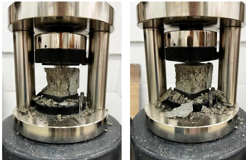
Figure 4.31 – Mortar Prism after Failure in the Compression Test.
