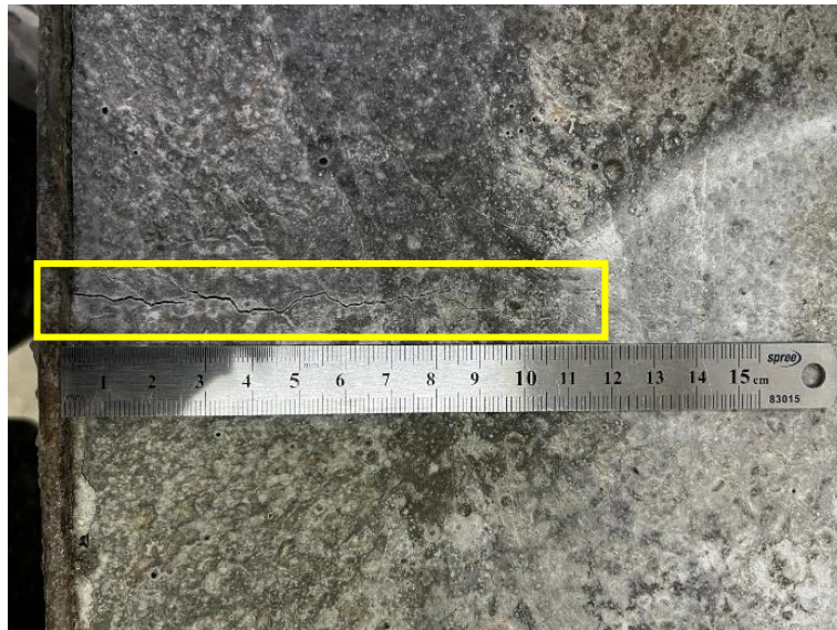
Figure 4.45 - Crack Formation above the Central Stress Riser in the Mould.
