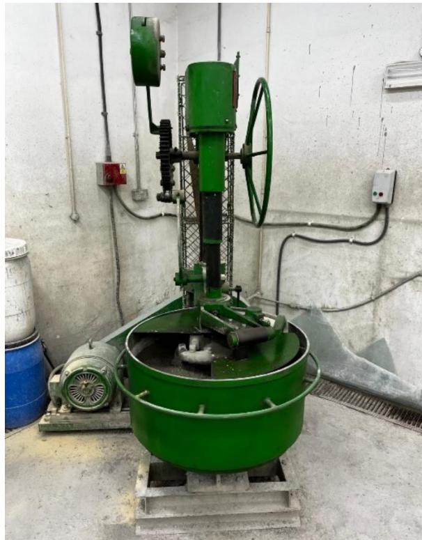
Figure 3.13 - Pan Mixer used for Casting all SCC Mixes.
