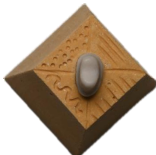
Figure 3.9 Improved prototype with smaller surface area for easier scanning, deeper grooves, irregular areas for landmark identification for best-fit superimposition and reduced tooth exposure to reduce surface area for scanning of die.
