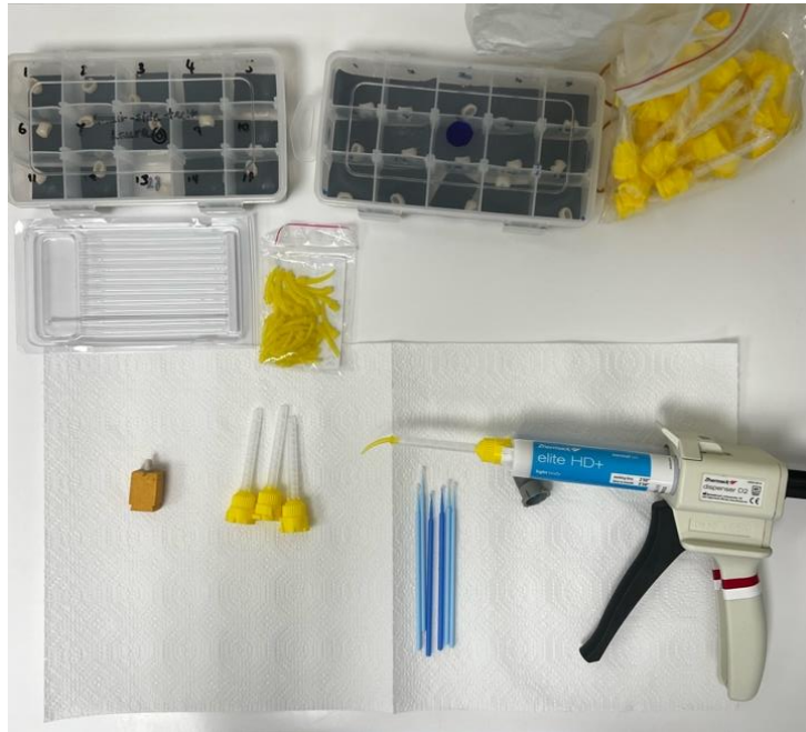
Figure 3.12 Scanning set up photo showing the two different crown groups in separate numbered boxes, the scanning aid and die, light body silicone material, micro-brushes and the adhesive tip for crown scanning.
