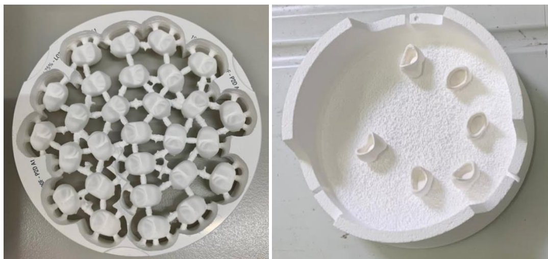
Figure 3.7 (Left) Zirconsahn Prettau 2 A3 blank with the milled crowns before removal of attachments. (Right) After attachment removal and polishing of the zirconia crown in the green stage using listed burs, the crowns were placed on a sintering tray with a base of fine-grain sintering granules as requested by the manufacturer before undergoing conventional sintering protocol. Granule size: 0.4mm-1.0mm
