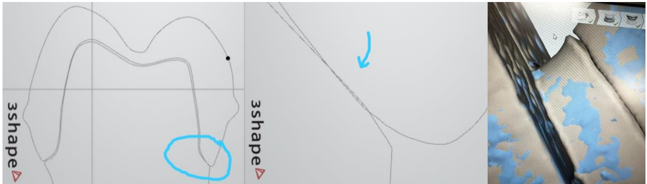
Figure 3.11 Screenshots taken using 3Shape 3D viewer showing overlap of meshes (left and middle). Marginal discrepancy visible after bite registration stage using the Trios 5 scanner directly after the scans (right).
