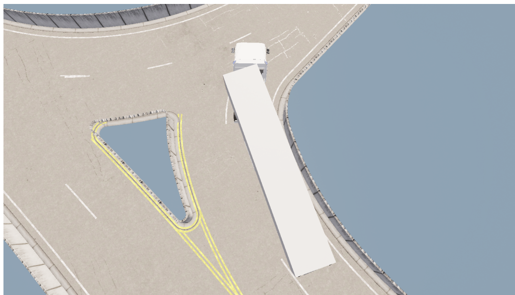
Figure 5.14 Trailer unit colliding with inside kerb during right turn on 50m roundabout.
