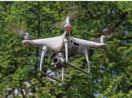
**Top left:** A typical drone used for aerial surveys
