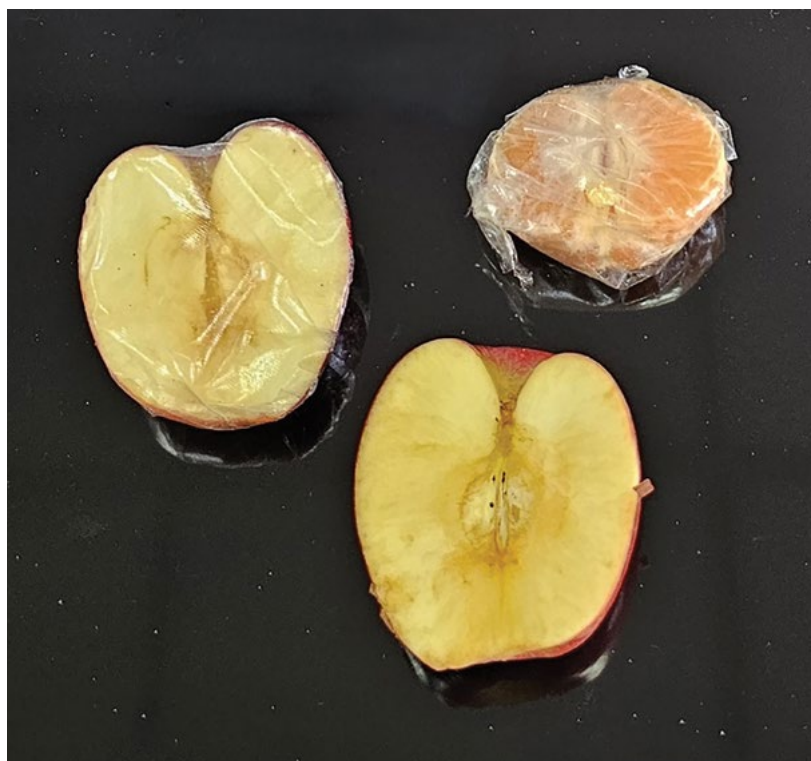
Testing biofilms covering fruit to show the real-life effects of the film. The covered apple is not as oxidised as the uncovered apple, even though they were cut for the same amount of time (approx. 5 minutes). The covered orange did not dry out after being exposed to air for 5 days.
