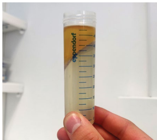
High-PUFA (polyunsaturated fatty acid) oils extracted and separated from waste Atlantic bluefin tuna Photo by Neil Cutajar
