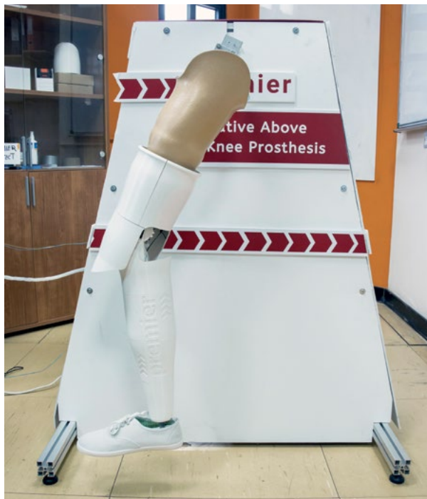
Smart above-knee prosthesis developed by Project PREMIER Photos by James Moffett
