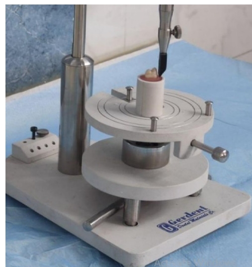
Figure 1 Mounting procedure: surface parallelism after acrylic pouring
