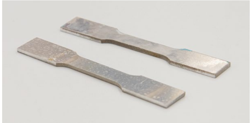
AZ80 magnesium alloy tensile specimens prepared for mechanical testing. Photo by Kristov Scicluna
