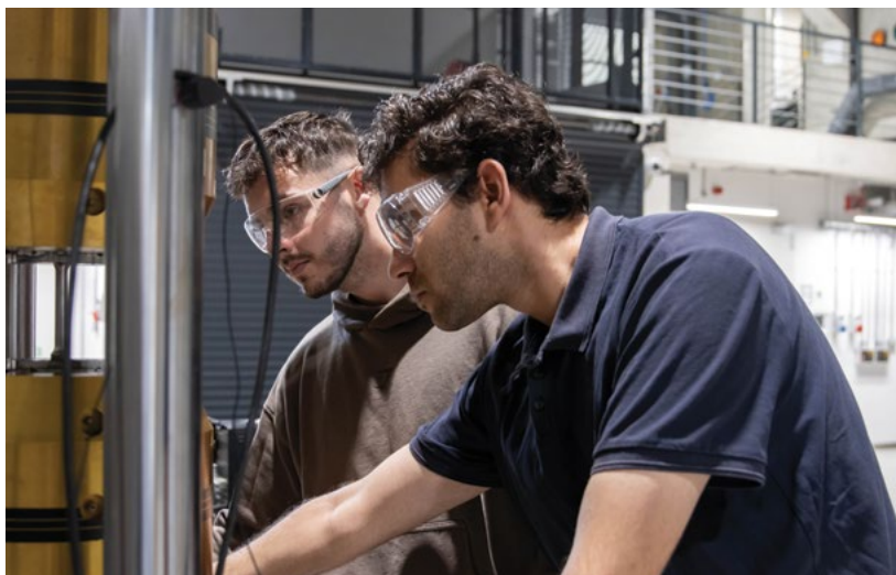
WAAMMS research support officers, Nejmeddine Layeb and Danjel Grima, running fatigue tests under cyclic uniaxial loading. Photo by James Moffett
