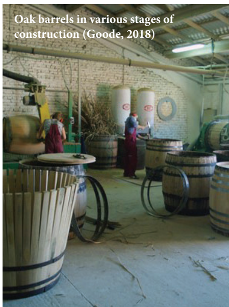
Assembling the barrel to the shape of a rose (Goode, 2018)
