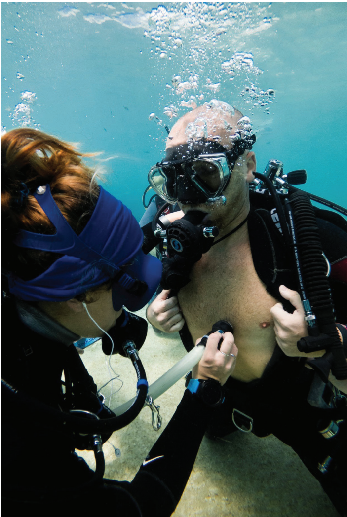
Microbubble flow measurement during a dive (with another prototype being tested in the process)
